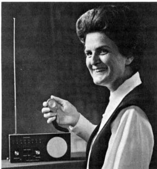
**This Bearcat fm scanner monitor has been converted to a transceiver by installing a Sonobaby fm transmitter inside. Many vhf-fm receivers have been used in this manner to build complete transceivers and walkie-talkies.**
