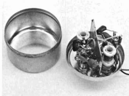
All wiring is done on the can's lid without the use of tie points.
