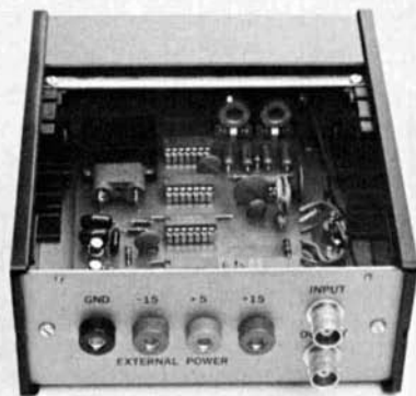
Rear view of the RY-170 AFSK generator with the top cover removed.
