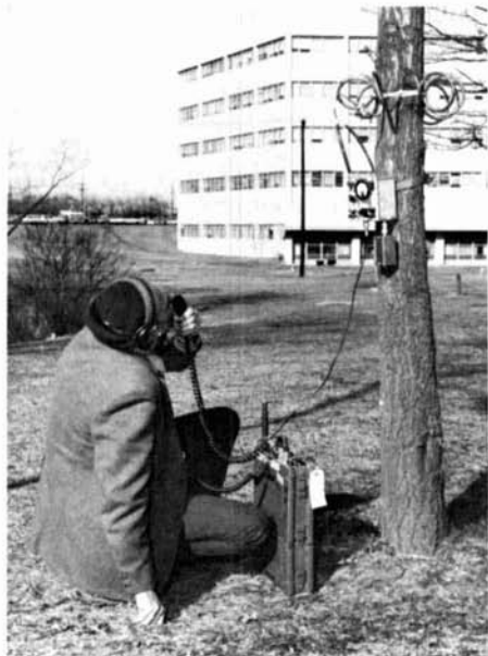
This tree is radiating a signal on 10.8 MHz. The transmitter is coupled to the tree through a matching network (in the box on the tree) and the toroidal Hemac. (U.S. Army photo.)
