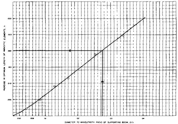
fig. 13. Supporting boom correction factor for the 15-element 432-MHz Yagi. Boom diameter is  $0.0275\lambda$  (3/4 inch or 1.9cm at 432 MHz); length of each parasitic element must be increased to  $0.2\lambda$ .
