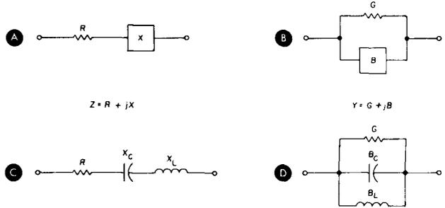
fig. 1. Rectangular form of impedance and admittance.
