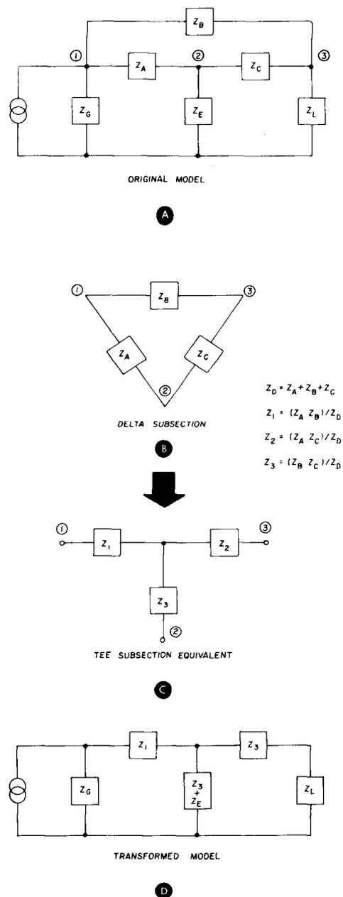
fig. 5. Model transformation. Here the delta subsection (consisting of  $Z_A$ ,  $Z_B$ , and  $Z_C$ ) is transformed into an equivalent tee section. The tee section is then added to  $Z_G$ ,  $Z_L$ , and  $Z_0$  to yield the transformed model.
