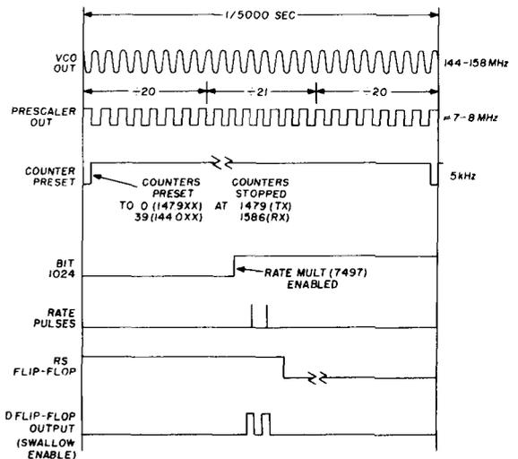
fig. 5. Programmable divider timing diagram. This diagram represents a frequency of 14X.X10 MHz.
