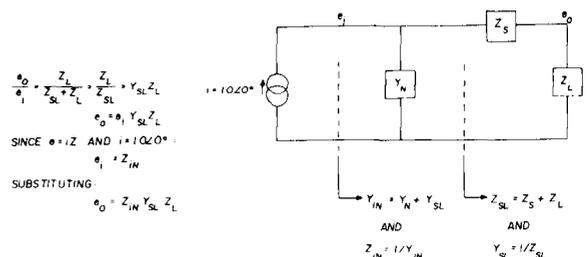
fig. 3. Basic model structure of the familiar pi network.
