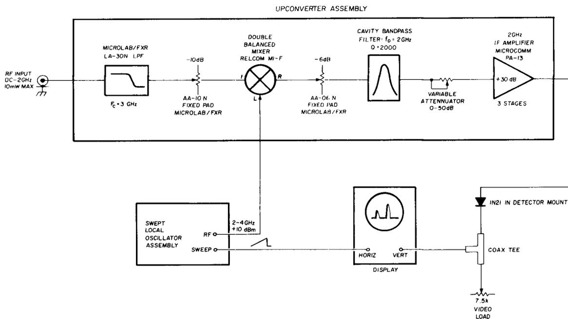
fig. 1. Block diagram of the microwave spectrum analyzer. Most components were purchased on the surplus market. The swept local oscillator, the key to the analyzer, is a surplus 2.4 GHz backward-wave oscillator. The display is an ordinary oscilloscope with dc coupling and provisions for external sweep.
