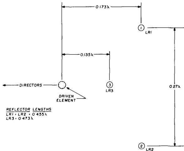
fig. 2. Trigrinal reflector arrangement (three reflector elements), when used with 4.2λ Yagi, provides 0.75 dB increase in gain (lengths not corrected for boom thickness).
