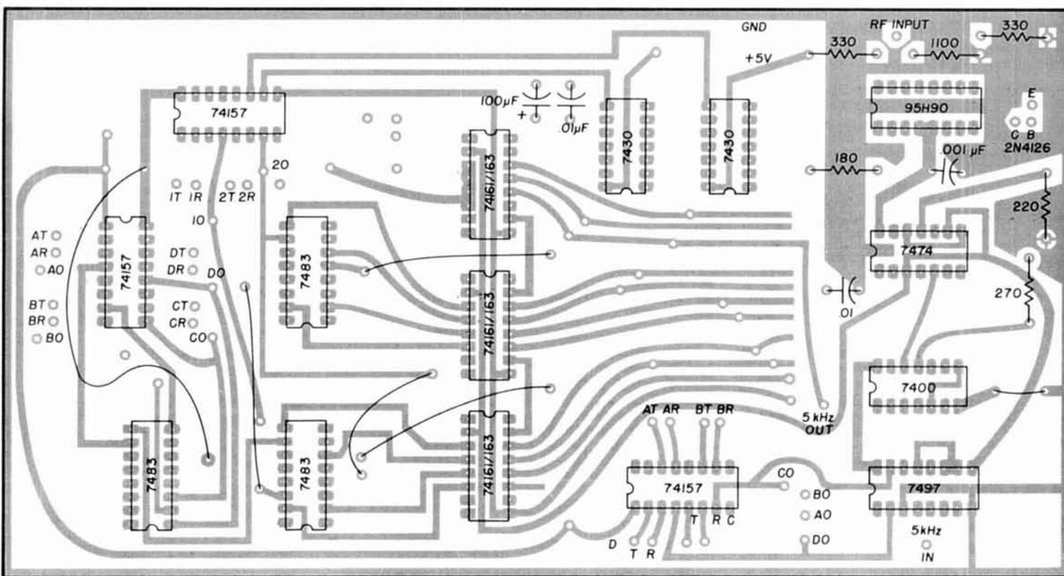
fig. 9. Component placement for the digital board.
