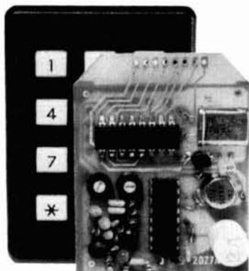
The 2027 dual encoder has both Touch-Tone and Sub-Audible tone on one small board. Simple installation in most radios requires only three connections: ground, plus VDC and tone output. The encoder itself slips over the pins of either a 12-key or 16-key DIGITRAN® keyboard.
