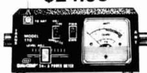
**Model 110 SWR/Power/Field Strength Meter.** Shows SWR from 1:1 to 3:1, RF power from 0-10 watts and 0-100 watts. Accuracy: SWR, 5%; Power, 10%. Frequency range: 1.5 to 144 MHz. Impedance: 52 ohms. Has 100 microamp DC meter, 5" bar antenna, SO-239 connector ..... \$24.95 plus shipping
