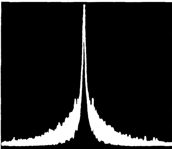
This spectrum analyzer photograph shows the output within 50 kHz of the center frequency. The 5-kHz sidebands can be seen to be 54 dB down from full output.
