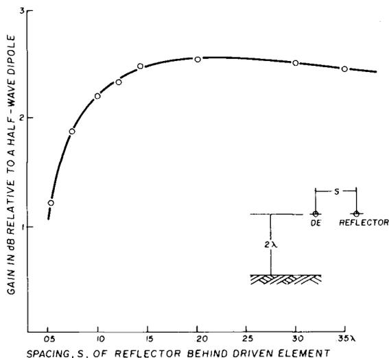
fig. 1. Gain in dB of a driven element and reflector for different spacings between elements.
