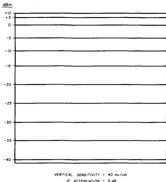
**fig. 5.** Typical vertical scale calibration of a spectrum analyzer with a logarithmic video amplifier. In this case display linearity is good at lower input signal levels, but compresses rapidly as the detector diode enters the linear region.
