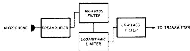
fig. 2. Block diagram of the logarithmic speech processor.
