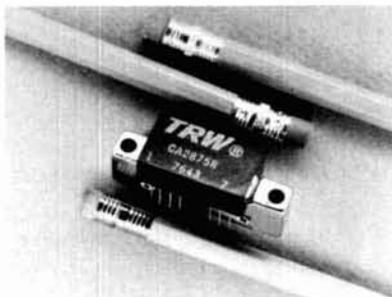
TRW RF Semiconductors has introduced an rf-hybrid gain block which will meet or exceed the most demanding requirements of i-f amplification in advanced microwave radio relay system applications.
