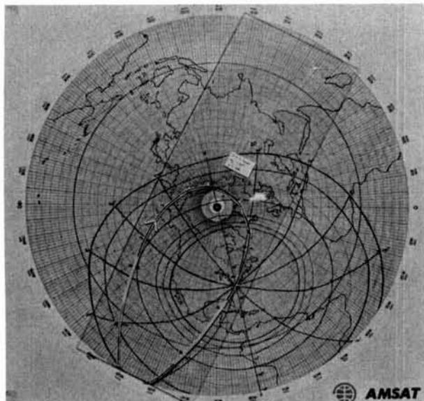
fig. 1. Photograph of *Satellable* style tracking nomograph for elliptical orbit of the type used by the Phase III-A spacecraft.
