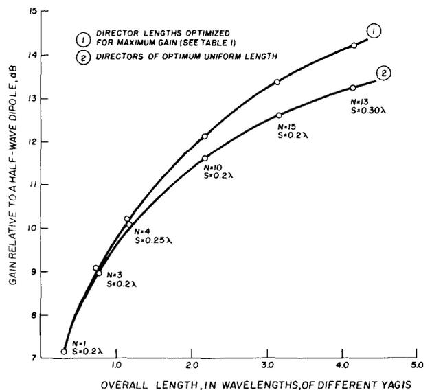
fig. 3. Gain comparison of different length Yagis, showing the relationship between directors optimized in length to yield maximum gain, and directors of optimum uniform length. *N* is the number of directors; *S* is the spacing between directors (reflector spaced 0.2λ on all antennas).
