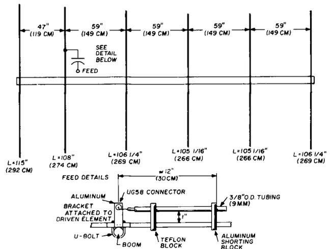
fig. 9. Layout of a 6-element Yagi for 50.1 MHz on a  $1.2\lambda$  boom. All elements are  $\frac{1}{2}$  inch (13mm) OD aluminum tubing, mounted on insulating blocks attached to a  $\frac{1}{2}$  inch (38mm) OD aluminum boom. The gamma capacitor is approximately 12 inches (30cm) of RG-8/U coaxial cable with the outer jacket and shield removed, then inserted in a  $\frac{3}{8}$ -inch (10mm) diameter tube.
