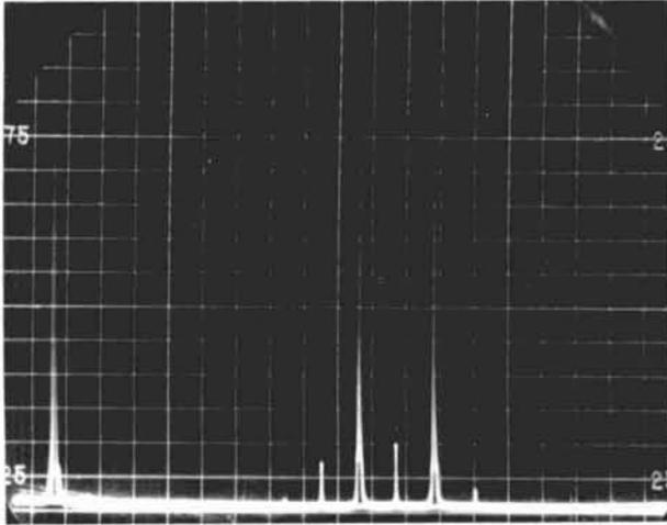
As a transmitting mixer's i-f port is overdriven, intermodulation products at  $LO \pm 2i-f$  become more pronounced, and the amplitude of signals at  $LO \pm 3i-f$  begins to increase. This display also shows the second harmonic of the i-f injection signal (at the left).
