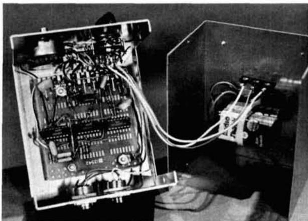
Breakaway section showing wiring and underchassis layout.
