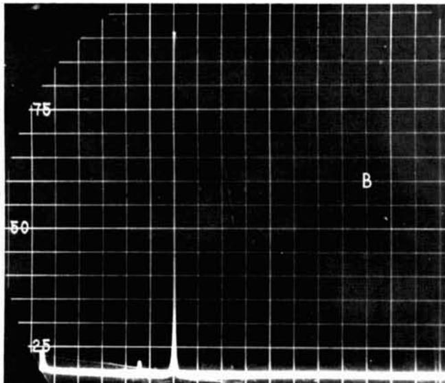
Example of spectral impurity, as displayed on the microwave spectrum analyzer. Presence of harmonic, subharmonic, and spurious signals shown in A is the result of an overdriven uhf amplifier. The same amplifier, with drive reduced to the rated level, is shown at B; the one spurious component is down by more than 20 dB. Display is from dc to 2 GHz.
