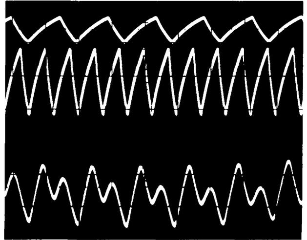
fig. 3. Addition to the low-tone oscillator (top trace) and the high-tone oscillator (center trace) to give a two-tone output signal when the digit 2 is pressed.
