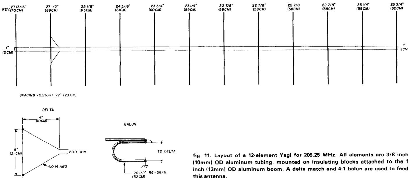
fig. 11. Layout of a 12-element Yagi for 205.25 MHz. All elements are  $3/8$  inch (10mm) OD aluminum tubing, mounted on insulating blocks attached to the 1 inch (13mm) OD aluminum boom. A delta match and 4:1 balun are used to feed this antenna.
