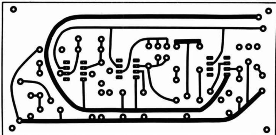
fig. 4. PC board layout, foil side.
