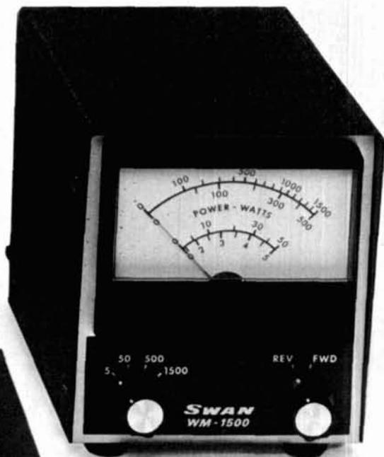
**Double-duty in-line wattmeter.** Use this meter for output power measurement and troubleshooting, too. Better than 10% full scale accuracy from 2 to 30 MHz, and you can go to 50 MHz with only slightly reduced accuracy. Four scales to 1500 watts and selector for forward or reflected power.
