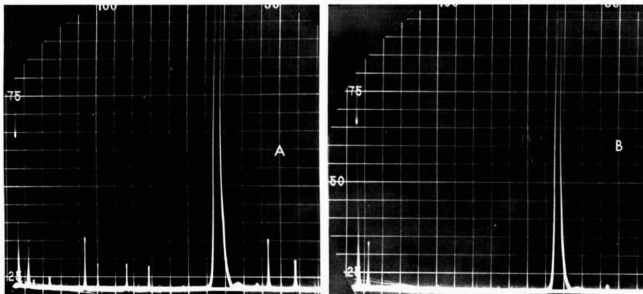
Output of a local-oscillator chain for a 1296-MHz converter. At *A* the i-f gain of the spectrum analyzer has been increased to show the spurious signals, which are 30 dB below the desired signal. The display at *B* shows the output of the same local oscillator after it has passed through a 3-pole bandpass filter. Although the filter has attenuated the desired signal by 1 dB, all spurious signals are down more than 50 dB.
