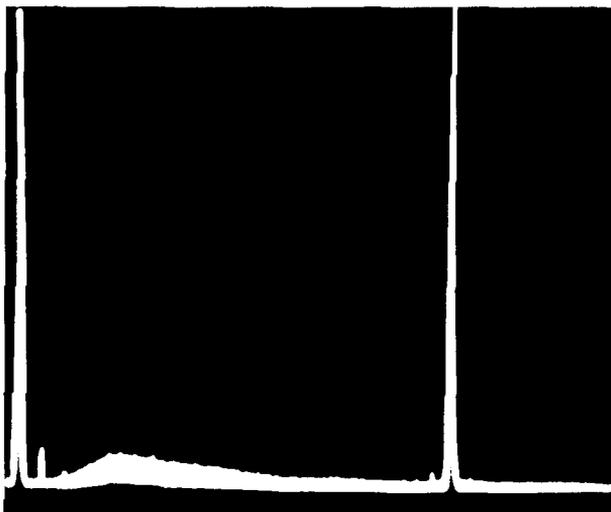
As shown on this spectrum analyzer photograph, the output is very clean from 0 to 200 MHz. The signal frequency is 146 MHz. The low-frequency noise is being generated by the rf amplifier on the rf board.
