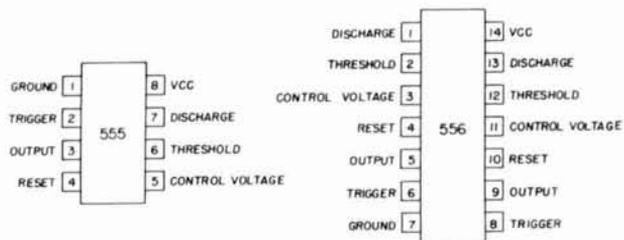
fig. 4. Pin-connection comparison for the type 555 and 556 timers.
