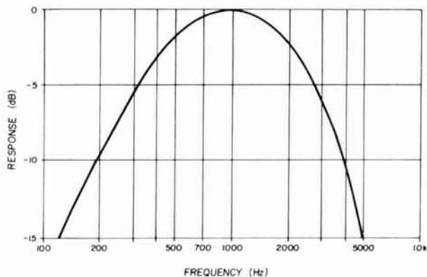
fig. 1. Speech-processor response below clipping level.  $V_{in} = 0.054$  volt p-p;  $V_{out} = 0.230$  volt p-p at 0 dB; Generator  $Z_{out} = 50$  ohms;  $Z_{load} = 1$  megohm.
