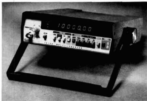
The Fluke 1910-A Multi-Counter is one of a series which provides frequency, period, period-average, ratio, and totalize functions. The 1910A is rated to 125 MHz; the 1911A and 1912A are similar in appearance and will measure frequencies to 250 and 520 MHz, respectively (photo courtesy John Fluke Manufacturing Company).
