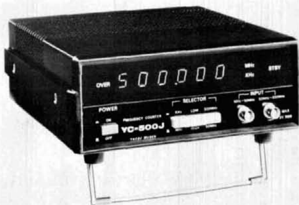
The Yaesu YC-500 Frequency Counter has a frequency range of 10 Hz to over 500 MHz. Its six-digit display provides the equivalent of eight digits when the gate time is switched. A room-temperature crystal, TCXO, or ovenized crystal time base may be ordered (photo courtesy Yaesu Electronic Corporation).
