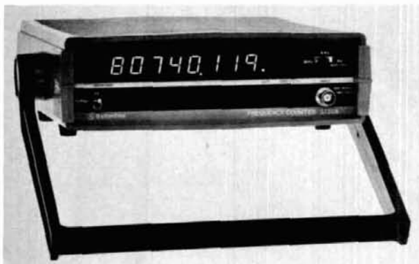
Ballantine's model 5720A Frequency Counter covers the range from 10 Hz to more than 80 MHz and provides frequency and ratio measurements. This counter also includes an audio multiplier circuit for input frequencies from 50 Hz to 1 kHz which provides resolution of 0.01 Hz with only 1-second measurement time (photo courtesy Ballantine Laboratories).
