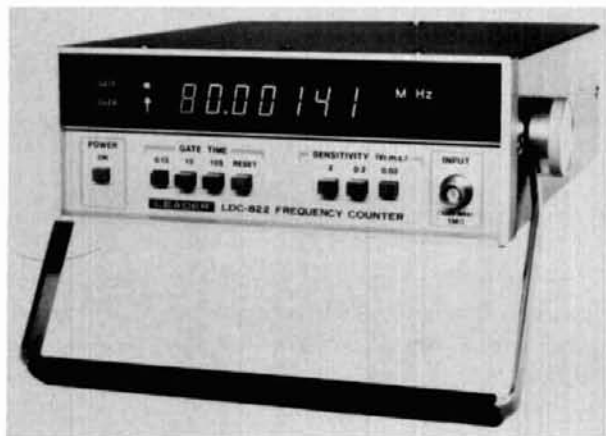
Leader LDC-822 Frequency Counter measures frequency to 80 MHz and features selectable gate time and input attenuation (photo courtesy Leader Instruments).
