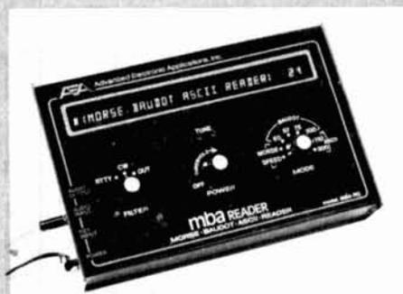
**What does MBA mean?** It stands for Morse-Baudot and ASCII. **What does the MBA Reader do?** The RO model (reader only) uses a 32 character alphanumeric vacuum fluorescent display and takes cw or tty audio from a receiver or tape recorder and visually presents it on the display.
