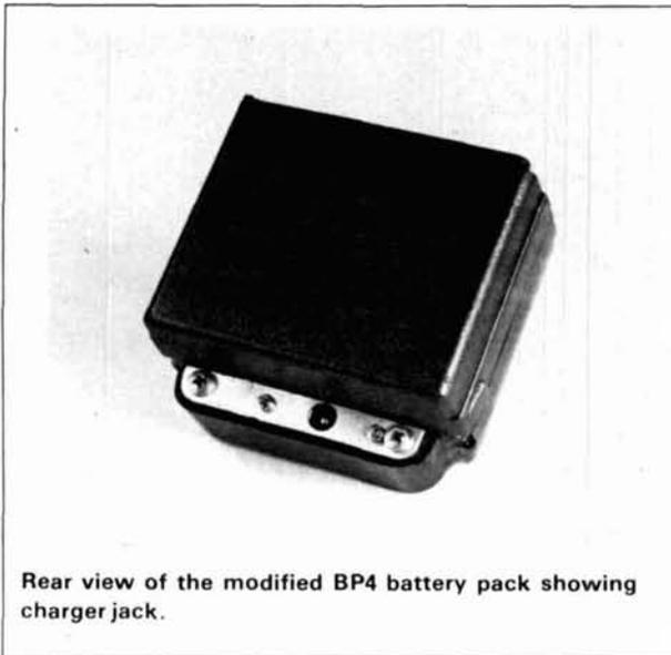
Rear view of the modified BP4 battery pack showing charger jack.
