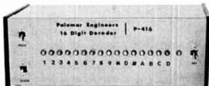
tor lamps show which digit is being received. Outputs will drive power relays directly and are either momentary or latched as selected by a panel switch.
