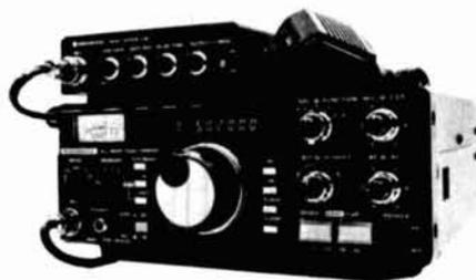
The rf output power is 10 watts on SSB, CW, and fm, and 4 watts on a-m. The Quad Bander operates on 13.8 Vdc drawing 1 ampere in receive, 4 amperes in transmit. Additional information may be obtained by contacting Trio-Kenwood Communications, P.O. Box 7065, Compton, California 90224.
