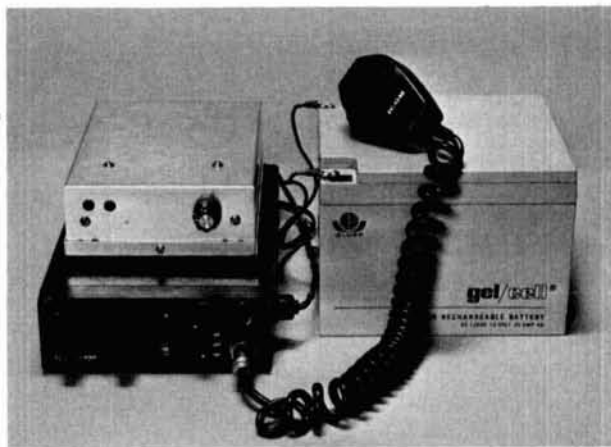
fig. 1. The Simplex Autopatch System. The autopatch controller is the small chassis on top of the ICOM IC-2302-meter transceiver. The battery is optional and allows continued operation after power failure.
