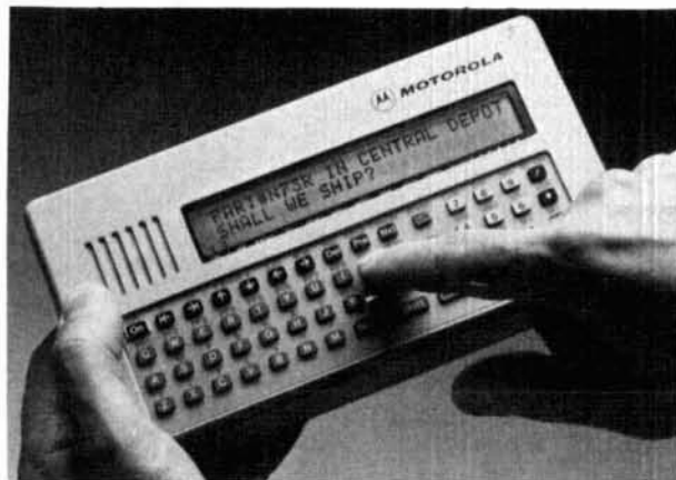
fig. 10. The portable radio data terminal (PCX) can provide interactive data communications with large data bases geographically dispersed. Thousands of such devices can modify inventories in real time, while roving around cities as part of area-wide packet networks operating in the 800-MHz business band. The local networks are in turn connected with a nationwide data network which provides updating of information to all other PCXs located elsewhere on the network. (Photo courtesy of Motorola Inc.)
