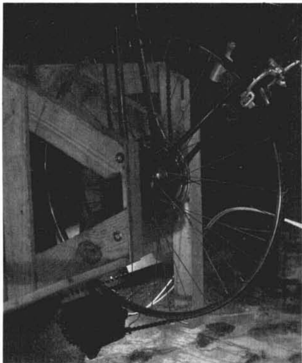
A length of ordinary cycle chain drives a ten-speed sprocket cluster mounted on the alternator shaft. The rear bike rim is wrapped in black friction tape and drives the chain like a large pulley. Crude perhaps, but the drive system is also inexpensive and mechanically efficient. (Photo courtesy W1GSL.)
