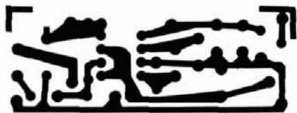
fig. 2. Full-size pc pattern is shown from the DIP side.
