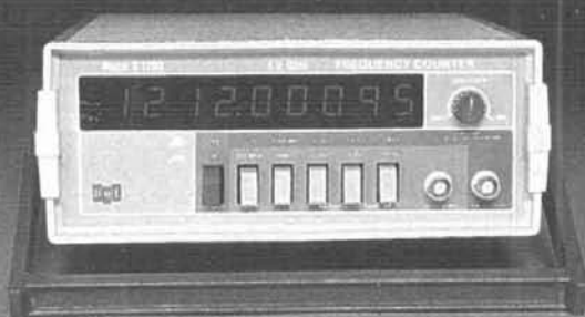
10 MHz Oven Oscillator 9 X 8 1/2 X 3 3/4 10 Hz to 1.2 GHz .1 PPM ACCURACY
