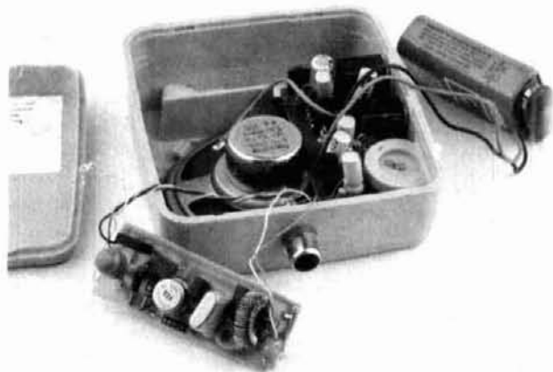
fig. 5. Few leads are needed to interconnect the rf board to the rest of the circuit.
