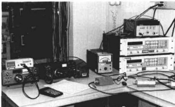
fig. 1. Laboratory setup used for testing the dynamic range of the two Argosys. The tests were performed with two tones at 14.020 and 14.040 MHz. Third-order product was recorded at 14.060 with the help of a true RMS voltmeter.
