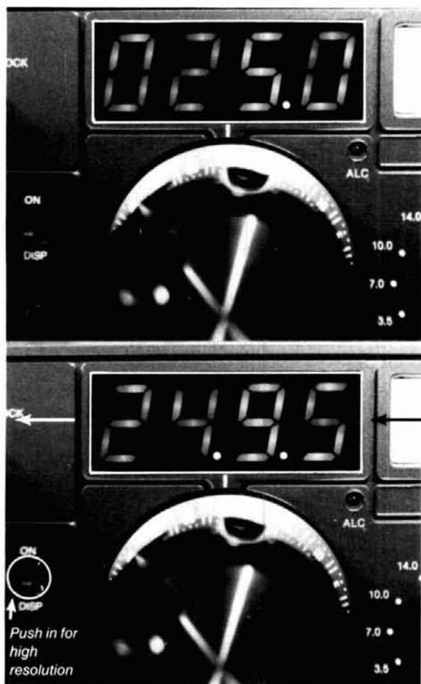
fig. 8. The Argosy frequency can be read to \pm 10 Hz (short term stability of the rig is fully compatible with this feature) by pushing in the "CAL" or "DISP" button on the front panel red windows. An additional decimal point will light up in the display (see lower view) indicating that the number has shifted to the left.
