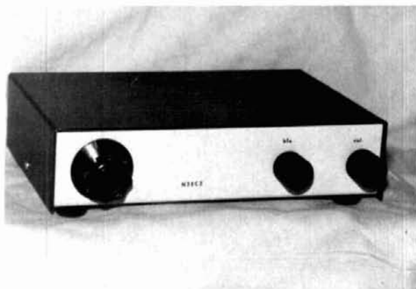
Photo A. The receiver cabinet measures 1 15 / 16 x 8 1 / 4 x 6 1 / 8 inch. (49 x 210 x 156mm). Main tuning knob is on the left. Lettering was accomplished with dry label transfers, and the panel was sprayed with clear acrylic.
