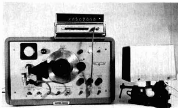
fig. 7. Measuring beacon frequency with an HP-540B transfer oscillator.
