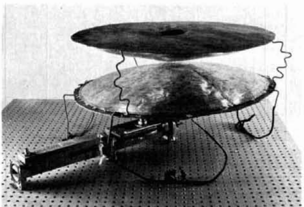
fig. 5B. Prototype X-band biconical horn.
