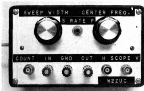
Photo 1. BP1 is labeled IN. Connect to input filter under test. BP3 is labeled OUT. Connect to output of filter under test.
