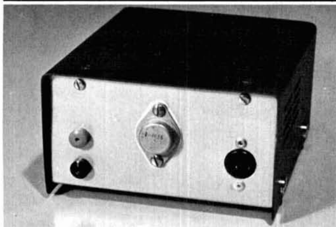
Back panel showing input jack and meter jacks. Q1 is mounted directly to the chassis (insulated if you wish) and requires no additional heat sink.
