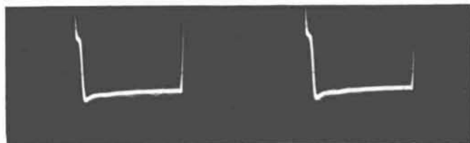
Same signal, same settings, except that the vertical position control has been changed.
