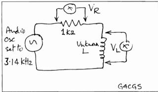
this reason the voltmeter used must be isolated from the audio signal generator. Insert the measured values into this formula and the result is in milliHenries:-
