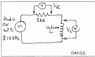
this reason the voltmeter used must be isolated from the audio signal generator. Insert the measured values into this formula and the result is in milliHenries:-
