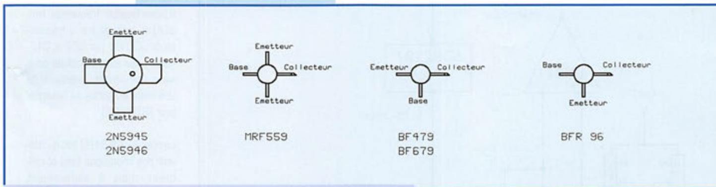
Figure 2. Brochage des transistors HF.
