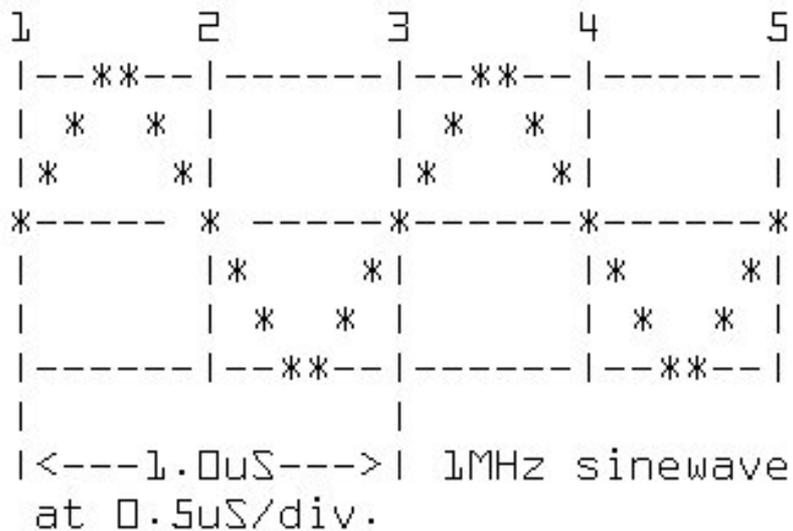
If you can't find the adjustment to tweak the horizontal gain, you can shrink or stretch out the test signal to the desired divisions using the HORIZONTAL WIDTH control, usually a front panel control. Then you can mark on the front panel where the HOR WIDTH control must be at each SWEEP setting for proper calibration.
