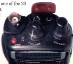
Fig. 4: Top of the C156. Here you can see the rotary knob (far right) which navigates the v.f.o. and memories, plus the extended menu options. Also you can see the 'VOLUME' rotary knob (middle) and the BNC connector for the helical antenna (left).
