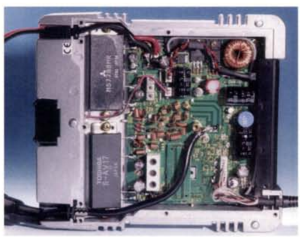
Fig. 10: Inside of the CPB510 'Power Booster'. (Top chassis view).
