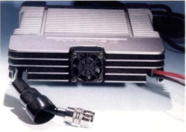
Fig. 9: The 'Power Booster' has a 'wander-type' coaxial lead terminating in an SO239 connector which has a built in duplexer (left).
