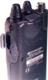
Fig. 2: The Standard C156 has the capacity to take the normal 13.8V d.c. external power and here you can see the connection on the left-hand side of the radio: 'DC IN'.
