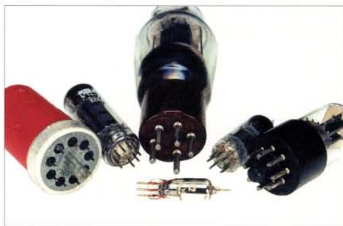
Fig. 1: Various valves and their bases. There are some fascinating valves around and the EF50 (left) was a pioneer used in Radar and has a remarkable history. Second from left is a B9A base ECL86 type, centre (top) is the famous 807 valve, and centre right a B7G based (incredibly versatile) EF91. Far right is a valve which uses the International Octal (IO) base. The diminutive valve below the 807 is a miniature type which found uses in everything from hearing aids to early 'hand-held' transceivers.
