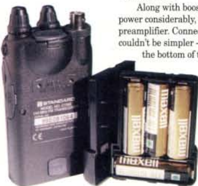
Fig. 3: The C156 v.h.f. f.m. hand-held Richard had for review was supplied with this battery pack in which he placed four AA cells. Richard said that he used normal alkaline batteries - 'cheapies' actually.
