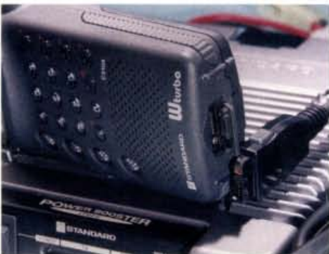
Fig. 8: Connecting the CPB510 to the C510 couldn't be simpler - a wander lead from the amplifier plugs into the bottom of the C510 hand-held and the C510 takes its power from the CPB510 which, in turn, is connected to a 13.8V d.c. power source by a standard plug.
