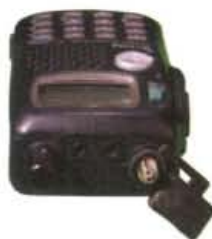
● Fig. 4: The top of the Icom IC-T81E. On the left is the rotary switch which controls the v.f.o. ranges and some other functions. In the middle you can see the 3.5/2.5mm speaker microphone socket and finally, on the right-hand side is the SMA antenna socket.
