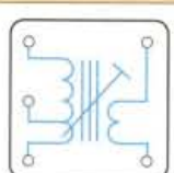
Pin out for the TOKO coil (please see 'Errors & Up-date' text).
