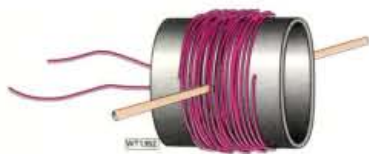
Fig. 4: A simplified drawing of the variometer L4. A glue gun was used to hold the winding in position and to secure the spindle where it went through the former.
