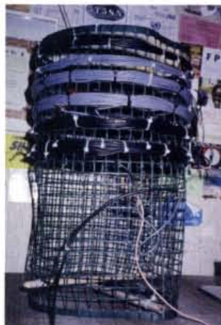
Fig. 2: The main coil, L1, standing on a 'spare' table in the shack. The distribution of the winding into 'bunches' and the cable ties can be seen.
