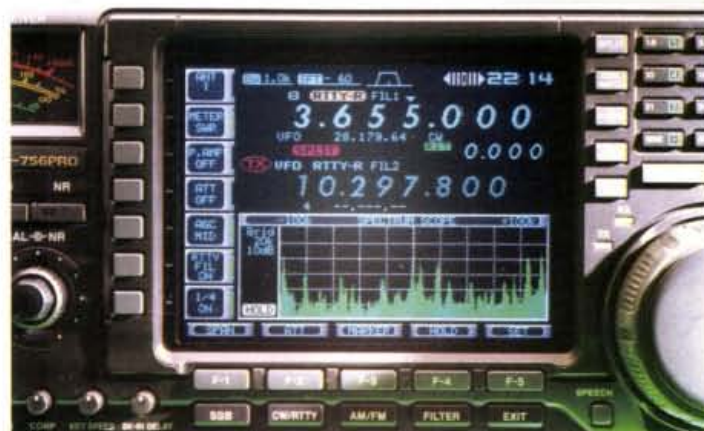
● Fig. 1: 'Looking in on frequency'. The main display on the Icom IC-756PRO provides a great deal of information plus a built-in RTTY screen (see text).
