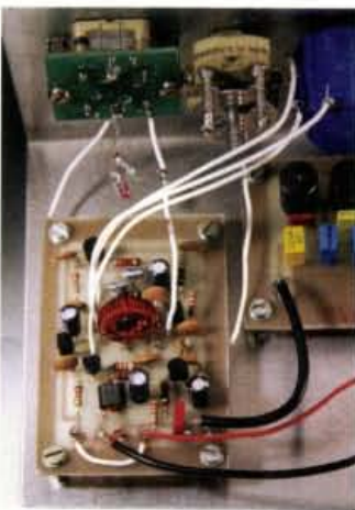
Fig. 5: Close-up of the main receiver p.c.b. of the receiver. The 'pig nose' ferrite bead transformer (described by G3RJV) can be seen mounted immediately to the left of the electrolytic capacitor in the lower centre of the p.c.b., just above the terminating coaxial connection (see text).
