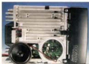
Fig. 4: Internal view of the top of the TM-D700E's main unit showing (amongst other things) the heatsink and speaker.
