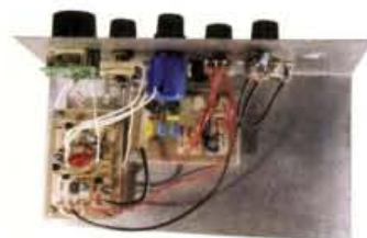
Fig. 4: An 'overhead' view of G3RJV's prototype receiver showing the layout and subsequent front panel controls (see text).
