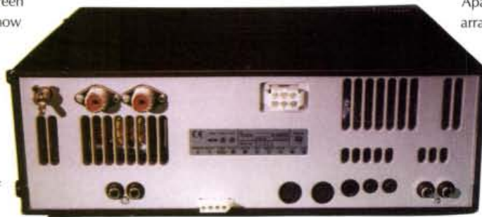
● Fig. 4: Photograph illustrating the rear panel of the Icom IC-756PRO transceiver. Unusually, this transceiver has a centrally-mounted panel with details of the various sockets, rather than having them individually marked.
