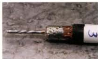
Fig. 6: Stage five, ready to fit the coaxial cable into the PL259 plug and solder them together. See text for an explanation.
