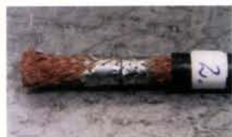
Fig. 5: Stages three and four of making a good connection to your PL259 plug. See text for an explanation.
