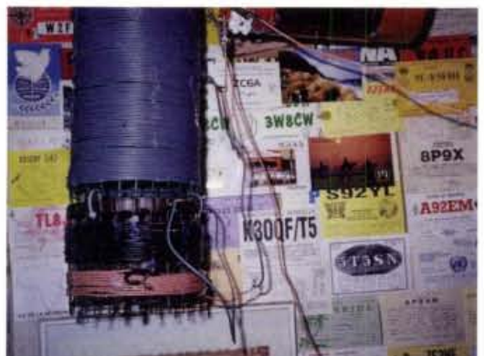
Fig. 3: Coil L2 which hangs vertically and to its right part of L3 can be seen. The variometer L4 is out of sight within the right-hand end of the coil former. On 2200m there's no advantage in having very short inter-connecting leads.
