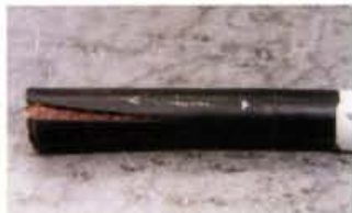
Fig. 4: Stage two of making a good connection to your PL259 plug. See text for an explanation.
