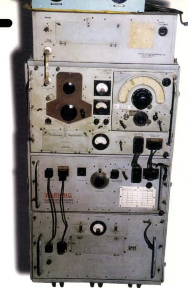
Fig. 3: The 53 Set transmitter. The power supply unit is at the bottom, with the modulator above. The r.f. deck is above the modulator, with the antenna loading coil at the top.
