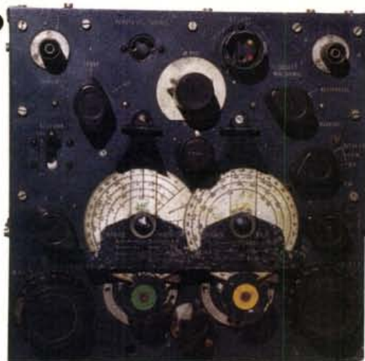
Fig. 2: The R1116 receiver, again, two tuning dials and very similar controls to the AR8 set.
