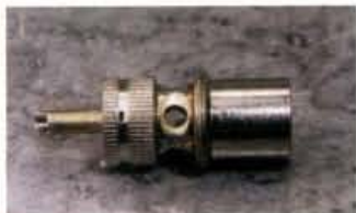
Fig. 3: Stage one of making a good connection to your PL259 plug. See text for an explanation.
