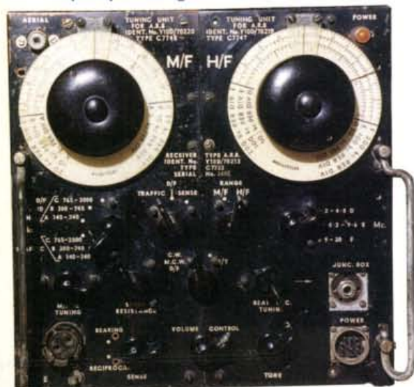
Fig. 1: The Australian AR8 receiver with the two tuning dials: low frequency on the left and high frequency on the right.
