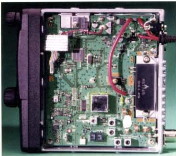
● Fig. 2: Internal view of the FT-2600. As Richard says, don't be fooled by its simple appearance, the FT-2600 offers full DTMF, DCS and CTCSS options and supports both 1200 and 9600bps Packet.
