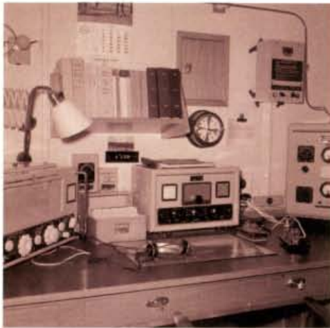
● Fig. 2: Radio station of MV Henri G/SLUR, 1959, showing main and standby receivers, part of emergency transmitter.
