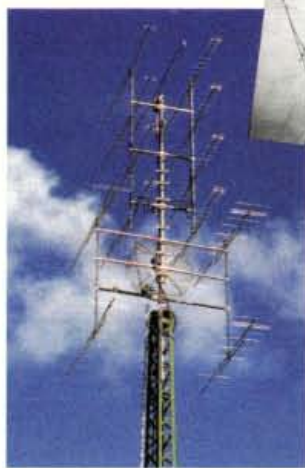
● Fig. 1: A four by two (stack and bay) set over a two by two set makes a reasonable e.m.e. set up on two bands.
