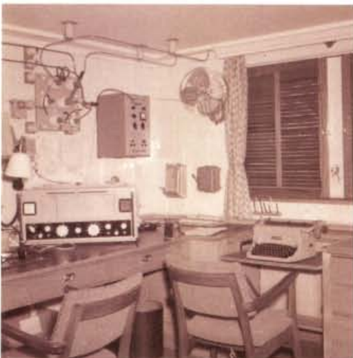
● Fig. 4: Radio station of MV Henri G/SLUR, 1959, showing main receiver, auto alarm receiver and antenna switch.
