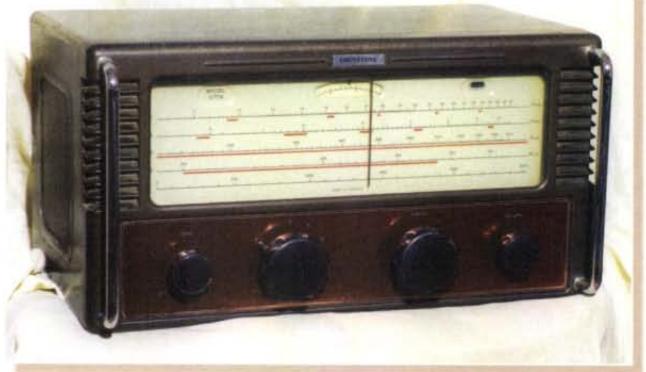
● Fig. 3: The Eddystone 670A receiver, modern 'B' styling but the same basic controls.
