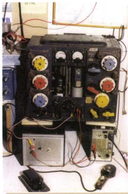
● Fig. 1: The T1154 in operation for the birthday bash. The 1000V h.t. and 6V l.t. supplies are underneath the set, the RAF 'Ground' or mains supplies couldn't be lifted into position as they weigh too much!
