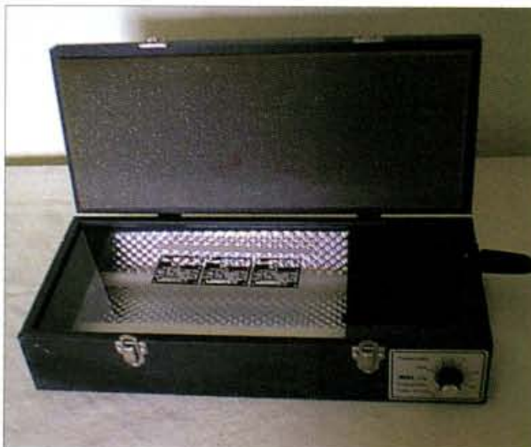
Fig. 1: An example of an ultra violet (u.v.) light box used to transfer the image to photo-sensitised p.c.b. material.
