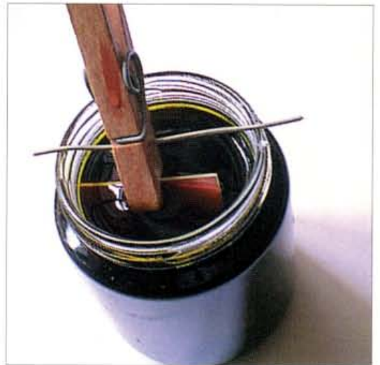
Fig. 2: George G3RJV's etching method - he leaves a small amount of unused space at one end of the board so it can be suspended vertically in the jar using a domestic clothes peg. A stiff piece of wire goes through a hole drilled in the wooden peg handle and this rests on the rim of the jar.
