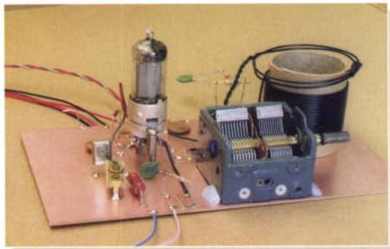
● No 'chassis' needed for this month's project - all you need for an 'old fashioned' circuit is modern printed circuit board laminate!
