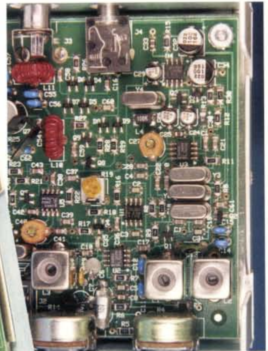
Fig. 1: Inside view of the complete MFJ-9340 (7MHz) QRP transceiver as built, by Clive Hardy G4SLU (see text for construction comments).
