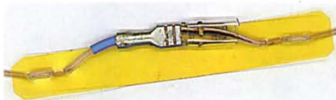
● Fig. 4: A cheap, simple and effective joiner for portable antennas.
