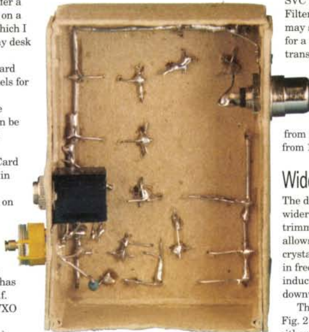
Fig. 3: Wiring the transmitter is exceedingly simple using the same technique for a p.c.b. lay-out. The whole assembly looks neat and innovative and will appeal to those of us who enjoy 'minimalist' radio construction!
