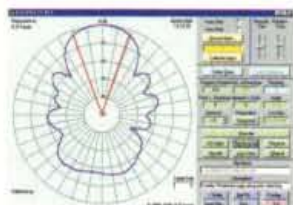
● Fig. 1: Antenna plots using the audio card on your PC are possible with a programs from Bob Freeth G4HFQ.
