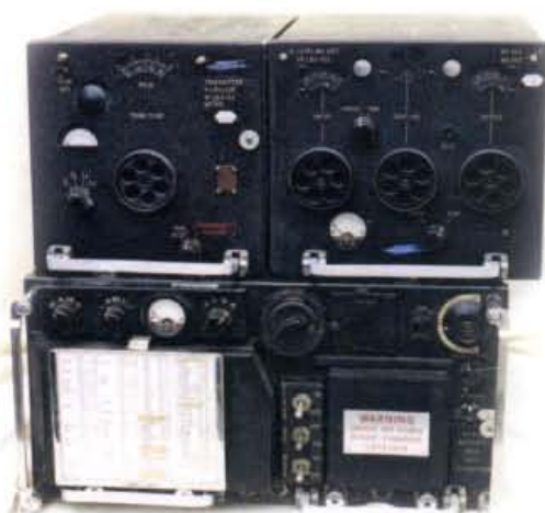
● Fig. 1: The STR18 units showing receiver/driver unit on the bottom, with the transmitter p.a. stage above left and the a.t.u. above right. The crystal controlled channel sockets are located behind the warning sign on the receiver (see text).
