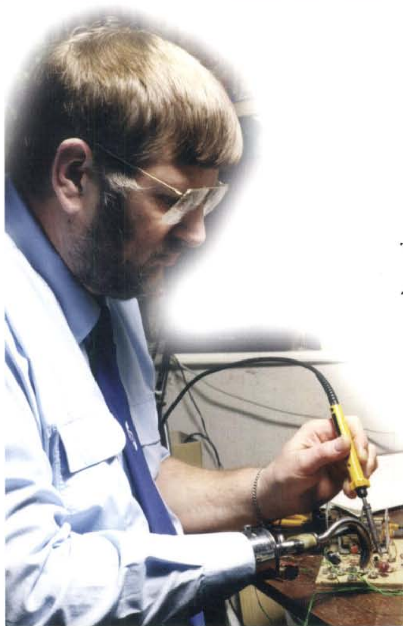
● Fig. 1: Rob G3XFD busy on his workbench using his Antex 25W soldering iron on a 'Radio Basics' project. Note his 'built in' heat sink and 'needle nose' pliers!
