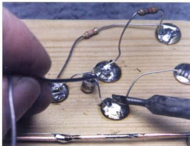
● Fig. 4: With care, once you have 'tinned' the top of the Drawing pin you'll be able to solder several points on to the pin without melting the solder on the whole of the head, thus not affecting the other joints (see text).
