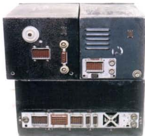
● Fig. 2: The rear of the STR18 units showing the various connectors, the 28 pin, 20 pin and four pin plugs and sockets, with Pye type r.f. connectors.
