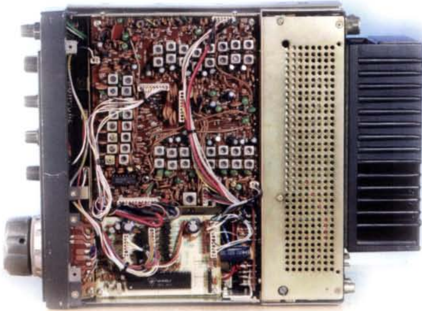
● Fig. 2: Inside view of the transceiver, showing the upper side of the main p.c.b. with relatively few integrated circuits and many discrete components.
