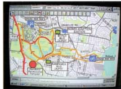
Fig. 3: The main APRS control screen. Amateurs were used to keep track of all the mobile TV units, helicopters and 'chase' vehicles during the Games. All tracking was done by APRS.
