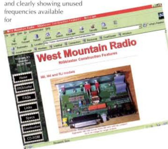
Fig. 1: RIGblaster connects your radio to your computer's sound card.
