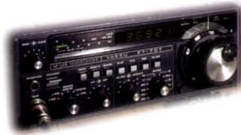
● Fig. 1: The neat front panel of the FT-707 transceiver. The main tuning display from the transceiver is provided by bright 'off white' i.e.d.s with a bar-graph type of indicator for power output indication. The digital frequency read-out is supplemented by a mechanical analogue dial counter. The neat and uncluttered control panel is exceptionally easy to use.
