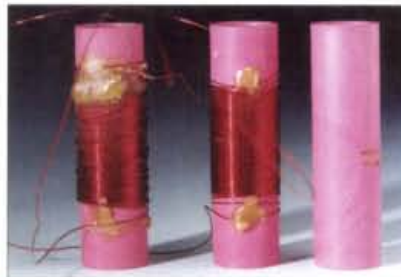
● Winding single layer and multi-layer coils. These were wound on plastic formers but the same applies for the paper tube former (see text).
