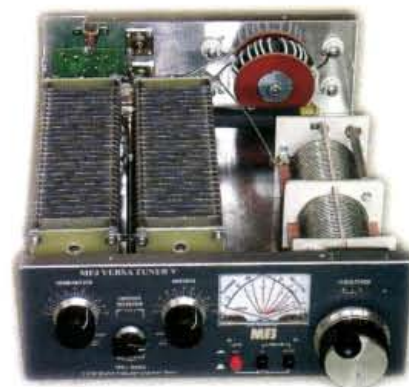
Fig. 5: Looking into the business 'bits' of the MFJ VersaTuner V.
