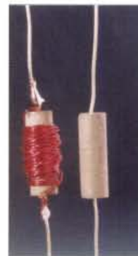
● Using a ferrite core with axial leads to wind radio frequency chokes (the cores are available from Sycorn).
