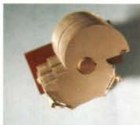
Fig. 6: Constant frequency capacitor (Note the offset turning centre).
