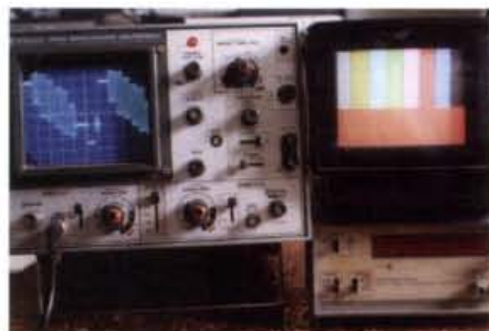
● Typical colour/bar/grey scale video test pattern as seen on oscilloscope and monitor. Frequency counter has a 50Ω input for direct measurements of low power transmitters.
