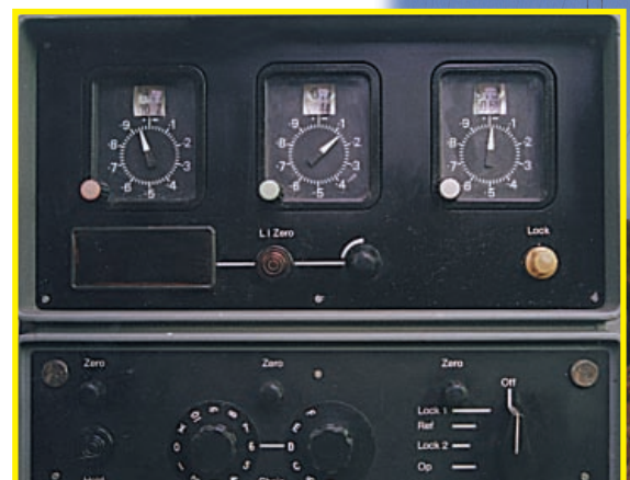
Fig. 4: The Mark 21 Decca Navigator receiver. The rectangle below the left-hand Decometer is the LI digital display which used Nixie tubes (see text).
