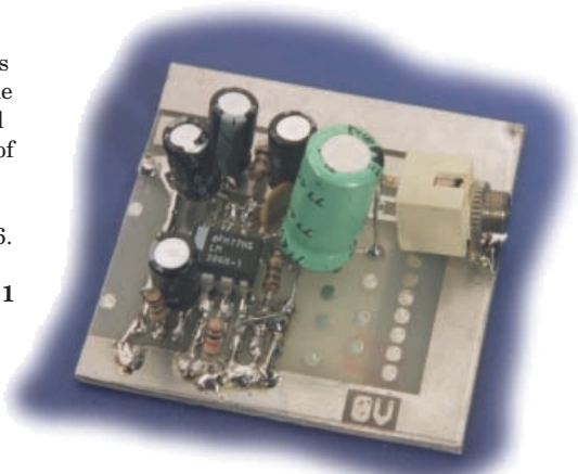
● Fig. 6: An audio amplifier built using the circuit featured in Fig. 4. George 3RJV says it works...but uses a lot of 100µF capacitors!
