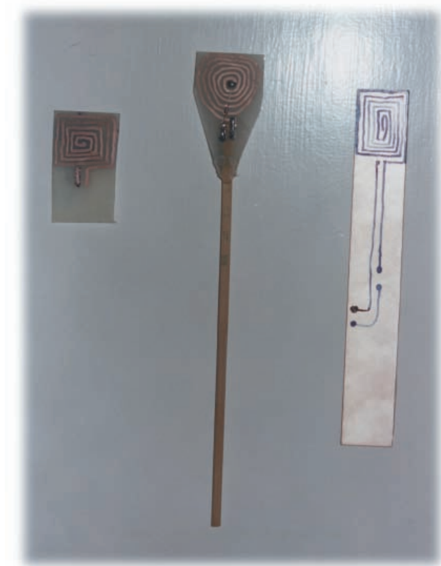
Fig. 2: Photograph of the RB Spatula project showing etched and un-etched designs. The p.c.b. design lay outs allows for the diode to be connected in circuit from the centre of the etched winding of the sensing coil to the meter connection (long strip p.c.b. version), thus providing the necessary link. Alternatively, the diode can be placed in circuit as shown in the version made using a hardwood handle (see text).
