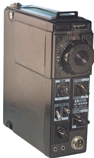
Fig. 1: Close up view of the front panel showing the simple controls on the crystal-controlled IC-202S.
