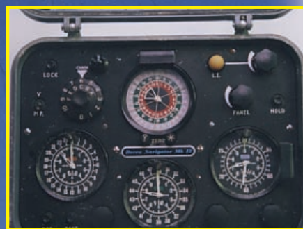
● Fig. 2: A mark 12 Decca Navigator receiver (see text).
