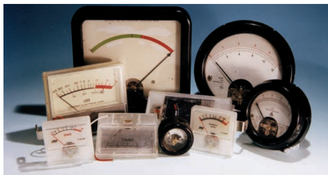
Fig. 1: Moving coil meter units galore! A selection of meters from the G3XFD and G1TEX collection. The large square meter at the rear (with right hand zero) was rescued from a redundant Band III v.h.f. 405 line television transmitter. The two large round types on the right are useful surplus units which both feature large single hole ring nut fixing methods (see text).
