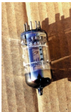
● Fig. 1: Phil 4JCP says "Take a look at a miniature valve and you'll usually find both a three-character code and a four-character code". The photograph shows the codes on a Mullard ECC81 (see text).
