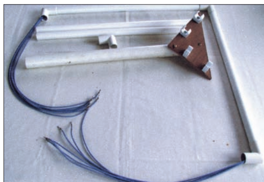
● Fig. 1: Part way in the construction of the loop. The wire bundle has only to be fed through the final two lengths of piping. The triangular plywood base is shown already fixed to the support pole using brass woodscrews.
