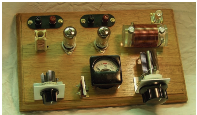
● Fig. 3: Johnny Apell SM7UCZ's v.f.o./p.a. 3.5MHz transmitter using two DL93/3A4 battery valves. The output stage draws a total of 24mA (18mA anode, 6mA screen) at 150V to provide an r.f. output of 1.2W (see text).
