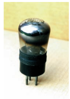
● Fig. 2: While rummaging through some old valves G4JCP came across a PM2DX - a 2V battery triode. It works a treat, but the filament draws 190mA at its rated 2V rather than the expected 100mA. Can you help solve the mystery (see text).
