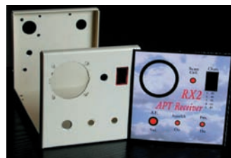
● Fig. 1: The start point after the front panel has the cut outs made, but before the new face panel is put in place.
