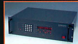
Antenna distribution units
