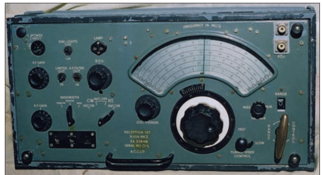
● Fig. 4: The British Army heavyweights R206 MkV reception set. The power supply plugs into the top left, and the large brass handle bottom right is the band change switch!
