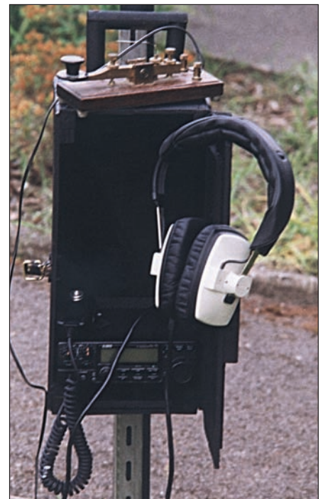
● Fig. 3: Using thin, very lightweight planed timber G3XFD made a box which will take one of the modern small h.f. transceivers (or home-brewed QRP equipment), an antenna tuning unit (a.t.u.), Morse key, headphones, wire for the antenna and radials, a gel battery, notebook and a small hammer.
