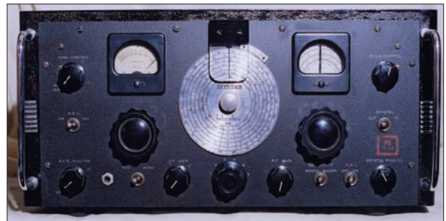
● Fig. 5: The Hallicrafters Skyrider receiver, an impressive looking, large black and heavy receiver. Ben G4BXD is looking forward to trying it out on the higher frequency ranges...a feature which made this receiver very useful during the Second World War for monitoring and test purposes.
