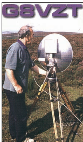
● Dave Hall G8VZT with portable microwave ATV.
