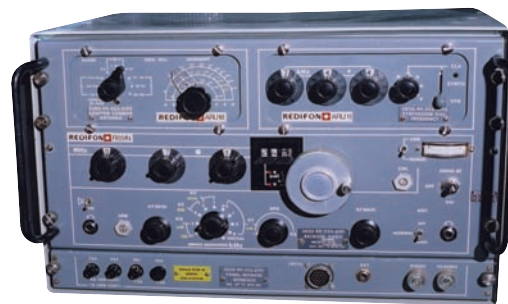
● Fig. 2: The Redifon R551N receiver, the synthesiser unit can be seen at the top right, and the a.t.u. at the top left of the photograph. The transmitter interface panel is along the bottom of the case (see text).
