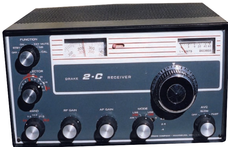
● Fig. 1: The Drake 2C receiver which has a clean front panel layout and easy-to-operate controls.
