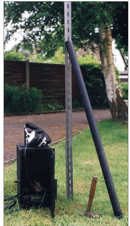
● Fig. 2: Although the box which you construct will be perhaps the most time consuming job entailed in making up your on PP system...other items are necessary. Rob has built his PP around the German made FTF fibreglass telescopic mast, which is supported by a lightweight length of angled steel (see text).
