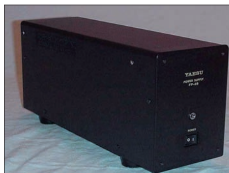
● Fig. 4: Power for the transceiver is provided by a switch-mode unit. This approach saves weight - especially for those special DXpeditions! (see text).
