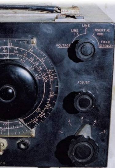
General Post Office (GPO)? It's obviously a field strength meter tuning dial, with the meter calibration for the unit?
