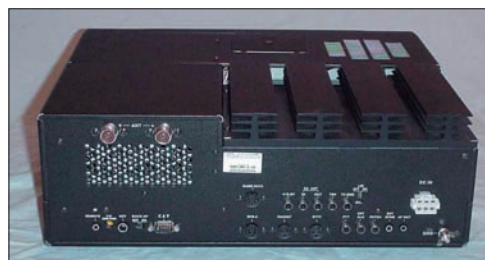
● Fig. 5: The rear panel on the FT-1000MP provides a host of connections for accessories and specialised operations, along with the two main antenna socket (see text for comments).
