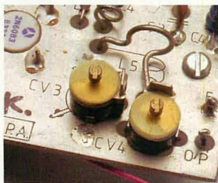
● Fig. 6: The so-called 'foil' trimmer, is relatively modern and can be regarded as a small air-spaced trimmer with thin polythene insulation. Delicate, although extremely useful (see text).
