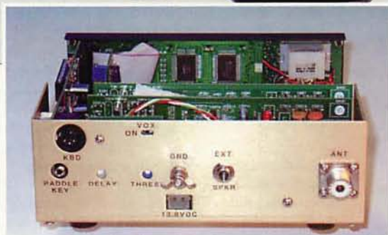
● Inside view of the Patcomm PC-500 15W transceiver (see text for comments).
