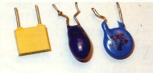
● Fig. 1: Commonly found capacitors. The type on the left is often encased in plastic, available in various values, often around 0.1 \mu F. A tantalum bead, resin dipped type is in the centre and silvered ceramic plate type encased in resin (right). See text.
