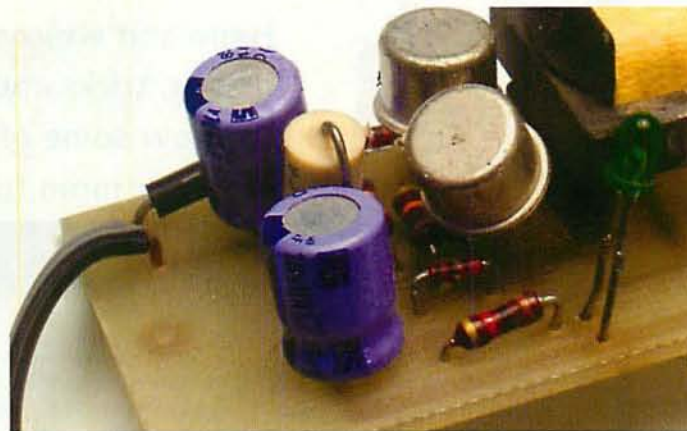
● Fig. 4: Modern sub-miniature larger value electrolytics, such as those on the left in this photograph, are very prominent nowadays. Modern circuitry has demanded their development. Although voltage sensitive they often provide anything up to 2000µF or more (see text).
