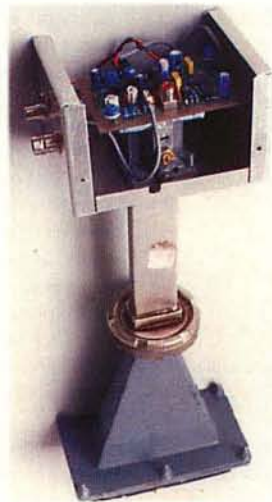
● Simple 3cm transmitter, showing Gunn diode modulator, waveguide feeder and horn antenna.
