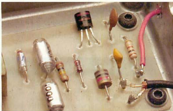
● Fig. 3: This form on the left of polystyrene/polythene coated, rolled silver foil/plastic dielectric type of capacitors, are the most likely types to give problems for beginners (see text).
