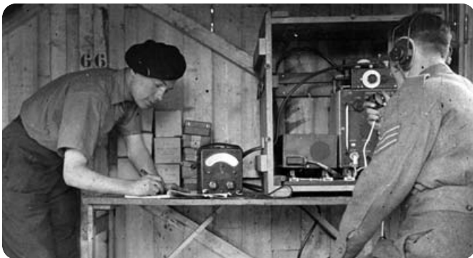
● Airborne S-phone equipment in use as a relay station in Holland during 1944-45. (Author's collection)
