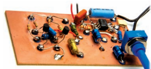
● One of the projects built by G3XFD - a multivibrator and audio amplifier unit (see text).
