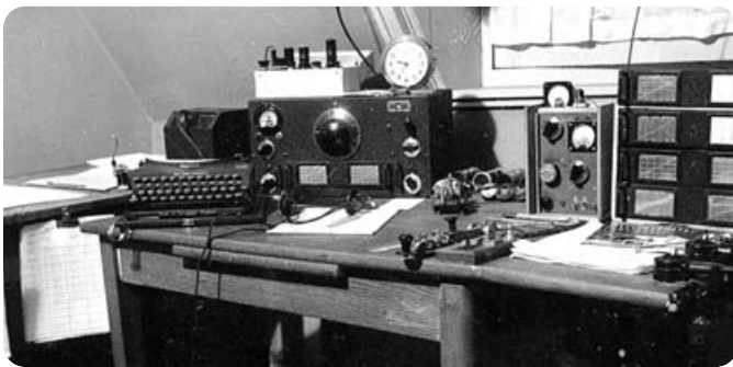
● An SCU9 station at Eindhoven, Holland, late 1944. Equipment includes a National HRO receiver, SCU Mark III (using 6V6 and 807 valves) transmitter and (on top of the HRO) the Mark VII/2 'Paraset' Agent transmitter-receiver which used 6SK7-6SK7/6V6 valves. (Author's collection)
