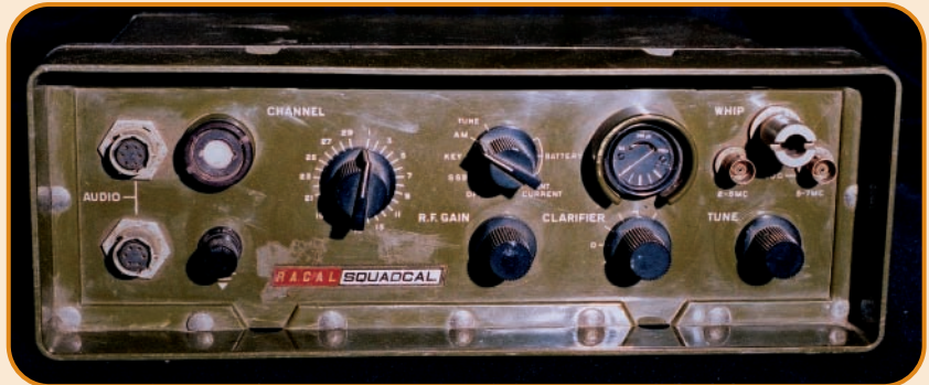
● The Racal Squadcal transceiver, a typical Racal plastic cased set (see text).
