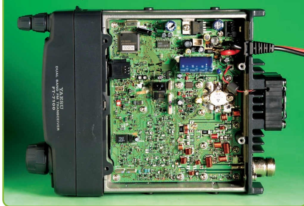
● Inside view of FT-7100M (top side of chassis view).
