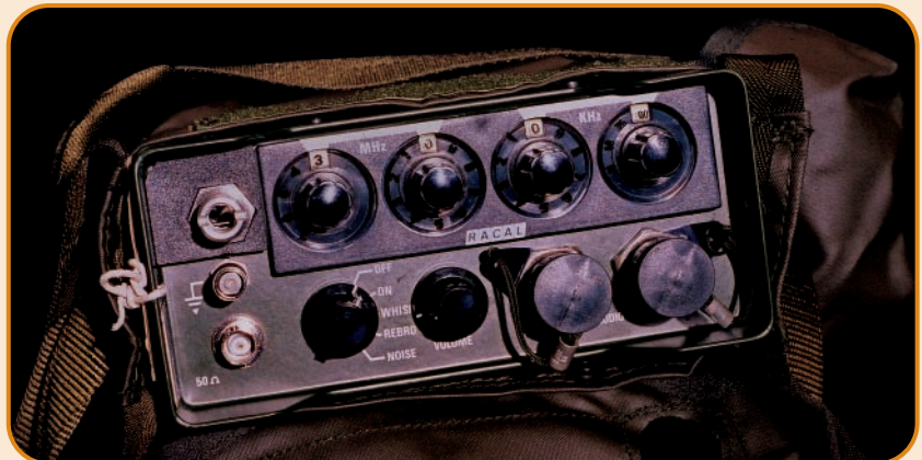
● The Racal TRA-967B in its carrying case. The four tuning knobs select the frequency in 25kHz steps (see text).
