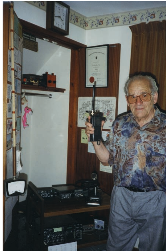
● Gordon G4VFV demonstrating an early prototype in action in the shack (hanging on the door, left) responding to the r.f. being radiated from the short helical antenna of a 144MHz hand-held transceiver.
