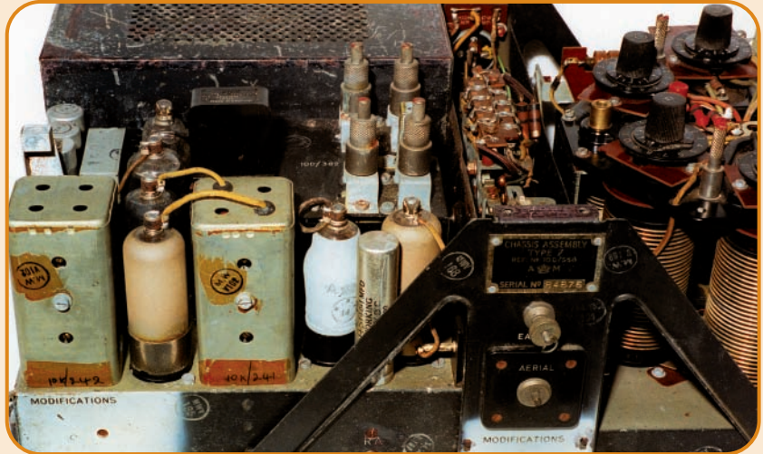
● Inside the TR-1196 receiver section, with the p.s.u. behind and the transmitter roller coasters on right.
