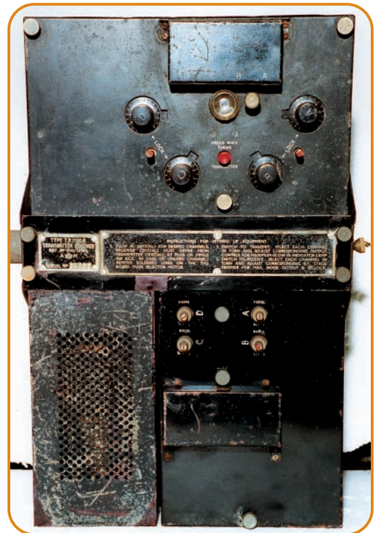
• The TR-1196 set, transmitter at the top, receiver on lower right with the power supply unit on lower left (see text).
