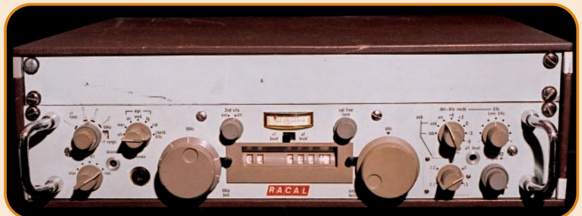
● The Racal RA-1217 receiver - rack mounting option - slim styling with fairly easy digital readout (see text).
