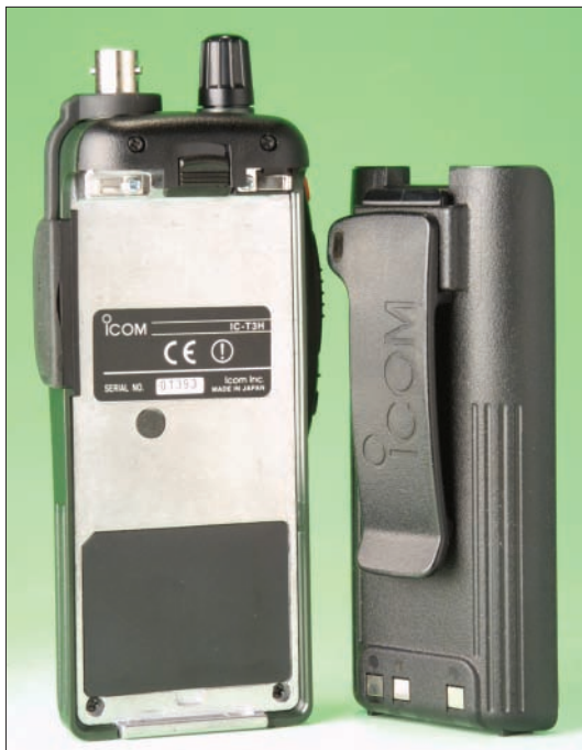
● Modern hand-held transceivers seem to be mostly battery pack! This view shows the battery detached from the transceiver (see text).
