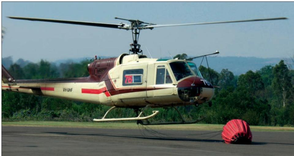
● Choppers like this one played a big part in trying to douse the flames of the recent Sydney bush fires. They are able to pick up up to 9000 litres (9 tons) of water in 45 seconds and then dump it onto the fires below!
