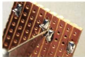
● Fig. 5: Running a strong knife blade between the tracks could detect, or even cure solder bridges. See text for details.
