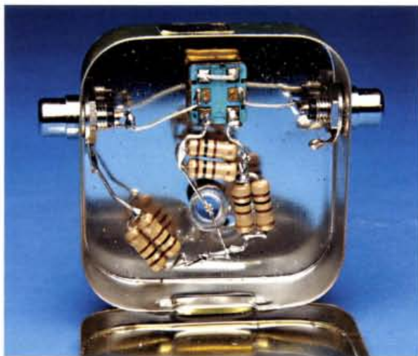
● Fig. 7: The simpler indicating bridge of Fig. 6 built into a small recovered metal box.
