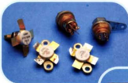
● Fig. 3: Specialised transistors - often used for v.h.f. and u.h.f. operations or power applications. The tabs provide power connections, input/output and form part of the heat-sinking and 'short lead' technology approach necessary for v.h.f. and u.h.f. applications.
