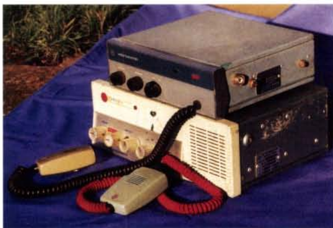
● Although the 70MHz band was originally popularised with the help of the surplus B44 transceiver, a large number of Amateurs used surplus converted commercial p.m.r. equipment (including G4JCP!). Pictured are two old favourites - the Pye Westminister (top) and Cambridge below (see text).
