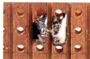
Fig. 4: A fine solder bridge (or hair) is shown here. This could cause the circuit to fail catastrophically.
