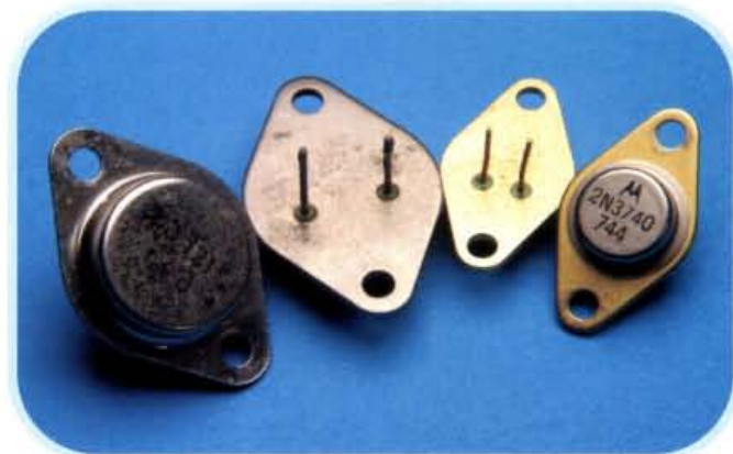
• Fig. 2: Older, but still useful power transistors. Often found in power supplies (where they are frequently used as current regulators) in older audio amplifiers and in car radios. General warning - some types can contain toxic chemical compounds. However, they are quite safe unless unsealed by filing or sawing.
