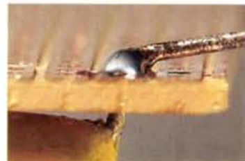
Fig. 3: The solder holds close to the edge of the track and could cause a solder bridge if another component is fitted in an adjacent hole.
