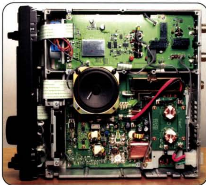
● Inside top view of the IC-7400.
