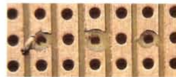
Fig. 1: Three examples of track breaks, only the middle one is correct, See text for details.
