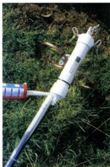
● Weatherproofing the matching unit prior to final assembly of the antenna (see text).
