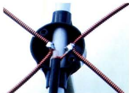
● Fig. 5: Close-up shot of the unbalanced feed connected to the 144MHz antenna.
