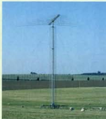
● Fig. 1: The RLPH steerable h.f. (6 to 30MHz) log periodic array. This antenna, although far from new is a valuable asset at the station. (photo courtesy of the RA)
