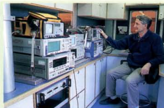
● Fig. 8: Inside one of the comprehensively equipped mobile labs. The monitoring equipment can be powered from an externally mounted generator or batteries. The ability to monitor waveforms and identify interference sources is paramount and the equipment is truly state-of-the art. (photo courtesy of the RA)
