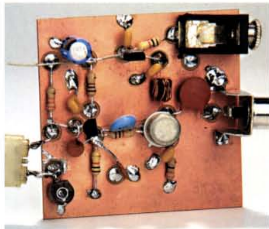
● You can build a 'bolt-together' transceiver - which you may be able to do immediately if you've already built the previously published projects! The 'OXO' shown here, is the heart of the design.
