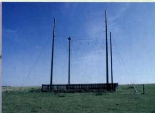
● Fig. 3: The calibrated cone antenna system, used by the monitoring station. (photo courtesy of the RA)
