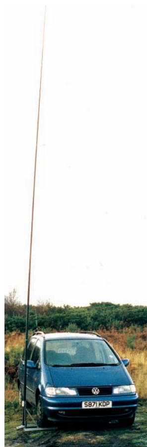
● Fig. 1: The Fibreglass 10m high telescopic mast in use with a Tenna-Tourer mast base (see text).
