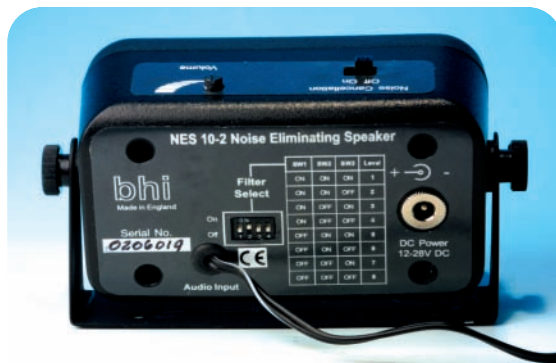
• Rear panel view of the NES10-2 unit. The DIP switch (just above the CE mark - provides eight levels of adjustment (see text).
