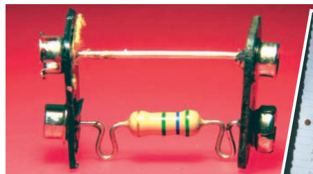
● Fig. 3: Steve VKAIM, suggests using older battery connectors as an adapter to make measuring current drawn easier.
