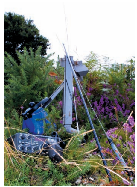
● Fig. 3: Some of the items G3XFD considers to be essential when operating 'portable! Firstly there's the kettle of course! Secondly, the trusty Trio 9000 multi-mode 144MHz rig, and Rob's 7MHz Pro-AM antenna, and a smaller h.f. whip. The sturdy metal unit in the background is the well-known Tennamast Tenna-Tourer drive-on mast base. This will support a lightweight metal mast up to 10m high, or one of the fibreglass 'fishing rod' type 10m masts available from PW advertisers Sycom. (A photograph of the Tenna-Tourer base in use with the Sycom mast was published in G3XFD's article - Delta Loop Portable on page 54 of the September issue).
