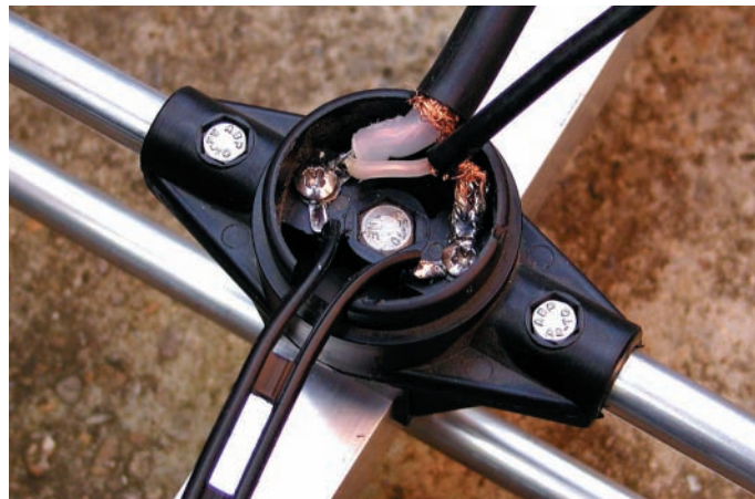
● Fig. 3: The cable entry box, before Neill G4HLX had discovered that the optimum match appeared to be with the coaxial stub removed! (See text).
