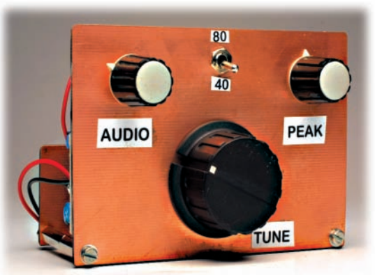
● This month’s project...a neat little 7MHz receiver based on the pioneering work of RA3AAE.
