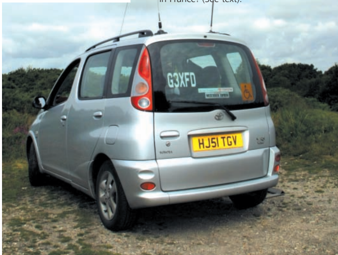
● Fig. 1: Rear view of the G3XFD 'travelling Amateur Radio station', showing the 144MHz whip (left) and the 7MHz Pro-AM h.f. whip (removed when travelling). The Toyota Yaris MPV is equipped for h.f. and v.h.f. operations. The internal lay-out of vehicle provides many 'nooks and crannies' for stowing equipment. The Yaris is fitted with air conditioning and is also provided with picnicking and tea & coffee making facilities (Well he does spend a lot of time driving!). And yes, the 'TGV' of the number plate was especially chosen...even though he doesn't try to race real TGV trains when in France! (See text).
