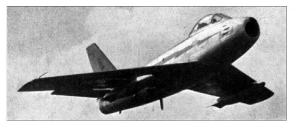
A North American F-86 Sabre It was fitted with a General Electric J-47-GE-27 pure iet engine which developed 5,800lbs thrust normally and 7,000lbs with water injection. It was capable of 680 m.p.h. at sea level and 630 m.p.h. at 35,000 feet. The service ceiling was 52,000 feet and the initial rate of climb 8,000 feet per minute. Compared with North American's famous P-51 Mustang this was pretty good, but not fast enough to catch a UFO!
