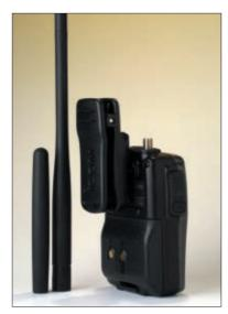
The IC-E90 and the two supplied antennas posed alongside the transceiver itself (the belt clip is shown attached to the transceiver). The IC-E90 does not have a function key to access an individual key's secondary job. Instead, all you need to do is keep a key depressed for a second or so to have instant access to the secondary feature. This makes one-handed operation much easier!
