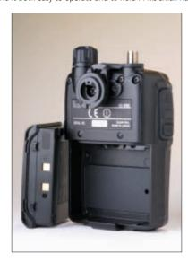
Rear view of the IC-E90, with the battery detached. The special moulded clip for the belt attachment (see text) can also be seen.
