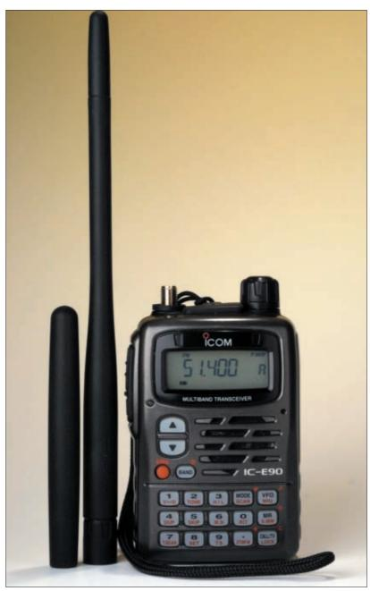
A transceiver and a general coverage receiver in the hand! Yes it's true...it's possible to transmit on 50, 144 and 430MHz and have extended receive coverage on both f.m. and a.m. modes from 495kHz through to 999.990MHz!
