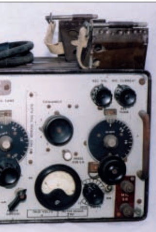
● Fig. 2: The war time Sound Ranging set, the controls are the same as used on the Wireless Sets 18 and 68 (see text).
