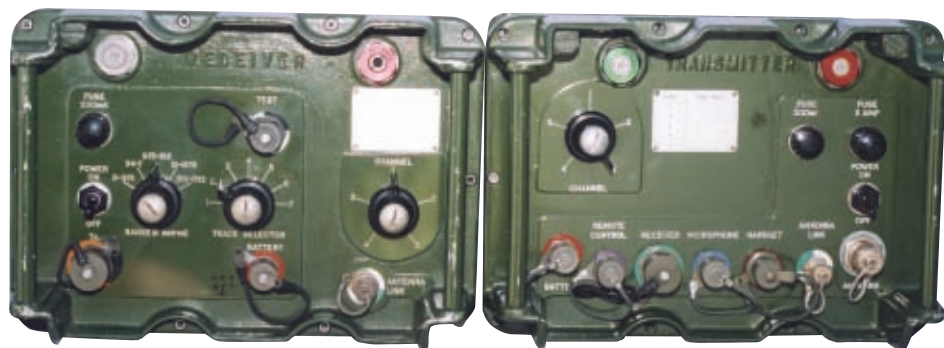
● Fig. 1: The modern Sound Ranging units, receiver on left, the transmitter on the right.
