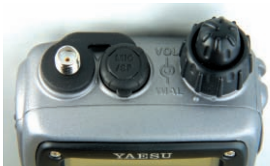
● A view of the top connections on the transceiver. Note the water-proofing precautions (see text).
