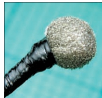
● Fig. 8: After trimming the foam and binding with electrical tape your microphone is ready for use.
