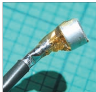
● Fig. 6: The bare home-made boom microphone.
