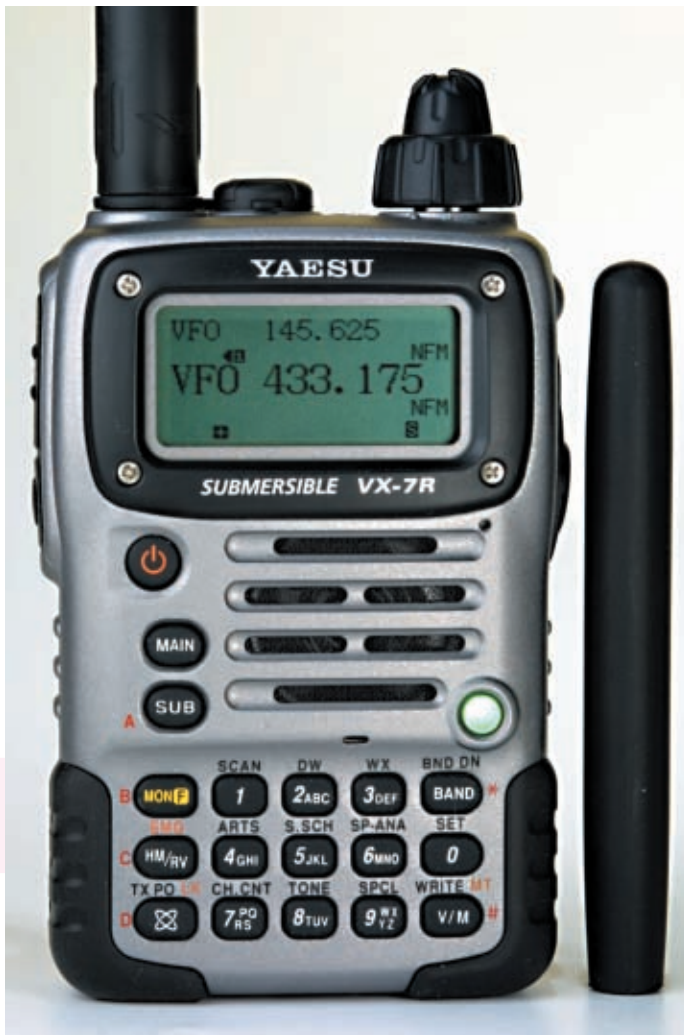
● A close-up view of the main front panel of the Yaesu VX-7R (see text).
