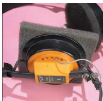
● Fig. 4: After cutting a piece of foam slightly larger than the earpiece, spray it evenly with a rubber photomounting glue. Allow it to dry a little before placing on the earphone and holding in place until fixed.
