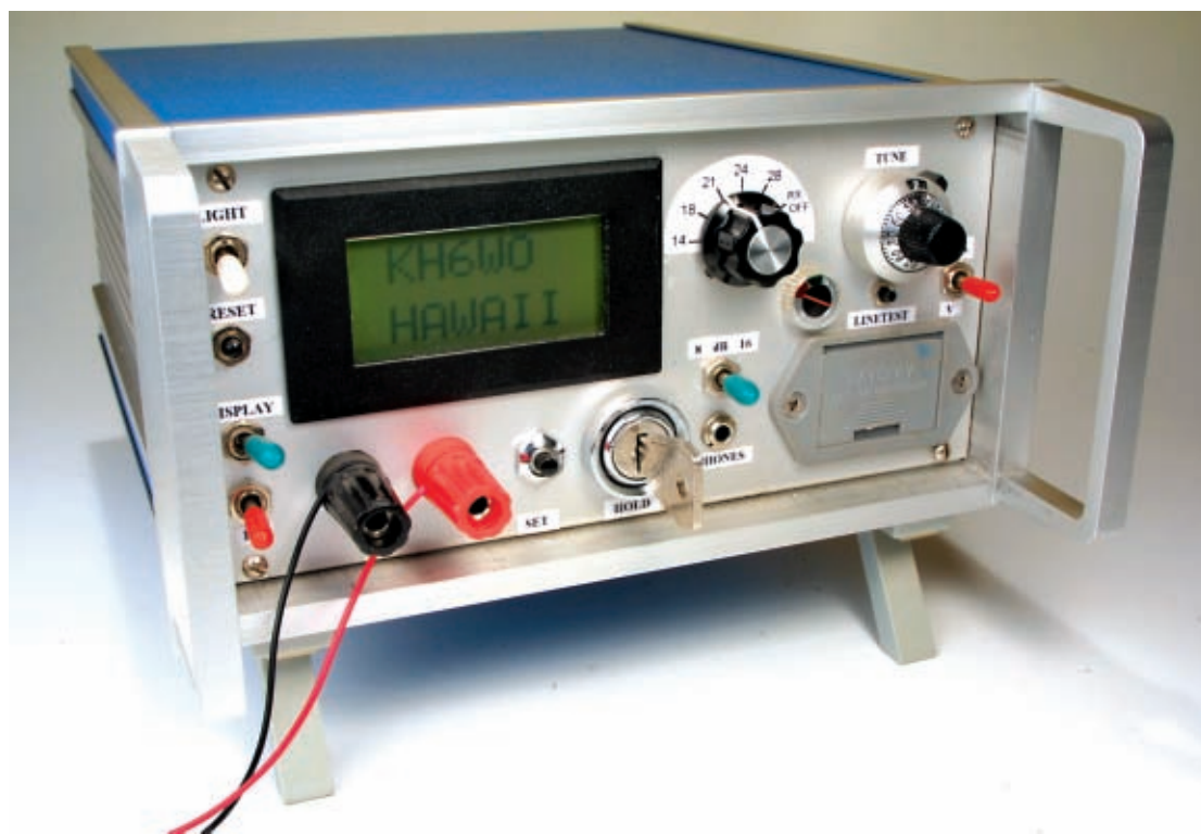
● The prototype PWIBP Monitoring receiver as built by its designer Oliver G3TPJ. This dedicated unit covers all five of the International Beacon Project frequencies on which the beacons operate, providing the operator with a means of evaluating band conditions within three minutes for each band (see text).
