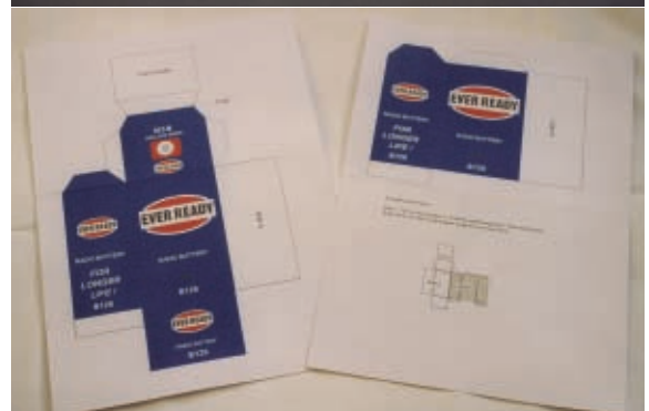
● Fig. 4: The power supply is built into the card case. Tony Westbrook, of the Kit Radio Company, has been experimenting with a laminated card case which incorporates a metallic screen (the flat, ready-to-assemble case is shown in here (see text).
