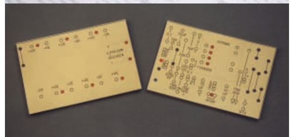
● Fig. 3: At first glance, the circuit boards look like conventional printed circuit boards. But they are in fact pieces of Veroboard with a printed overlay (see text).
