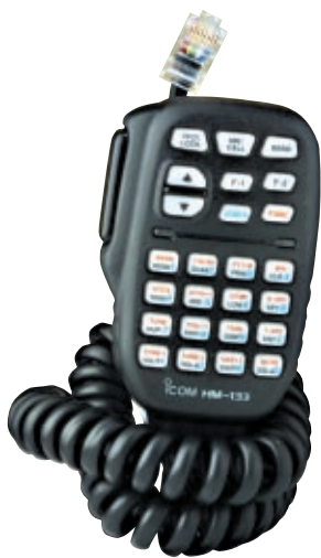
● The microphone with its comprehensive keypad, which facilitates the setting up of the rig and programming the memories (see text).
