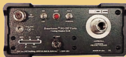
SG237 PORTA AUTOMATIC PORTABLE COUPLER
