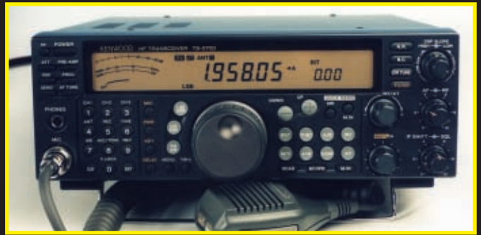
● Fig. 6: The Kenwood TS-570D transceiver which comes fitted with digital signal processing (DSP). This transceiver has an exceptionally large and clear main display (see text).
