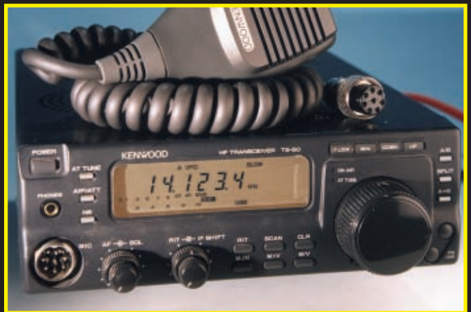
● Fig. 4: Another pioneer - the Kenwood TS-50 has proved to be an exceptionally reliable transceiver. The International Beacon Project system uses 18 TS-50S transceivers which operate 24 hours a day...seven days a week! (See text).
