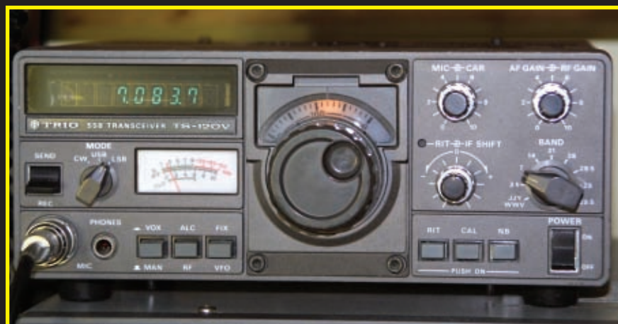
● Fig. 1: The Trio-Kenwood TS-120V low power c.w. and s.s.b. 3.5 to 28MHz (no WARC bands or 1.8MHz) transceiver. This 10W rig performs very well and is also extremely reliable. The photograph shows one in use in the shack belonging to Kevin Nice G7TZC/M3SWM, Editor of Short Wave Magazine .
