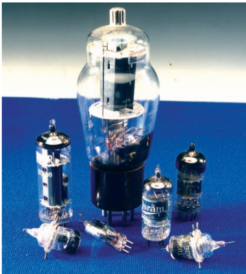
● Fig. 3: A variety of valves that were frequently used for home-brew equipment, from the larger 807 transmitter valve to the Acorn valves mentioned above.
