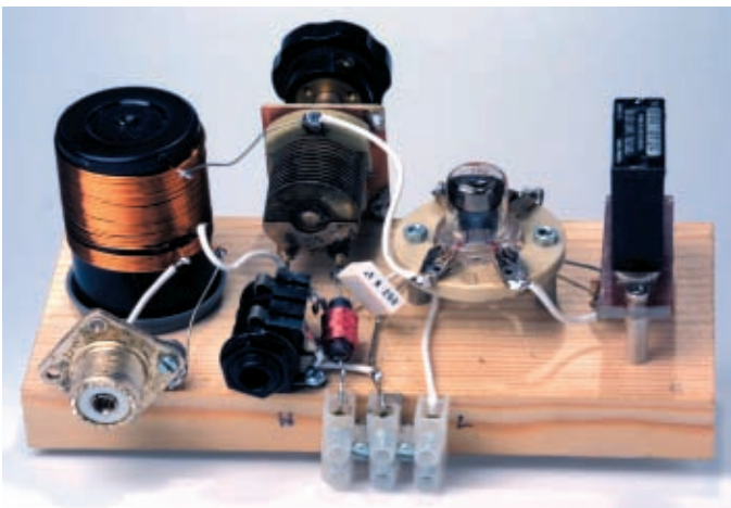
● Fig. 5: The Acorn valved transmitter, featured in the September 2002 issue of PW .
