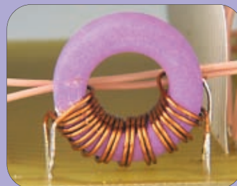
● Fig. 8: The 10-turn bifilar wound balun. (See text for details.)
