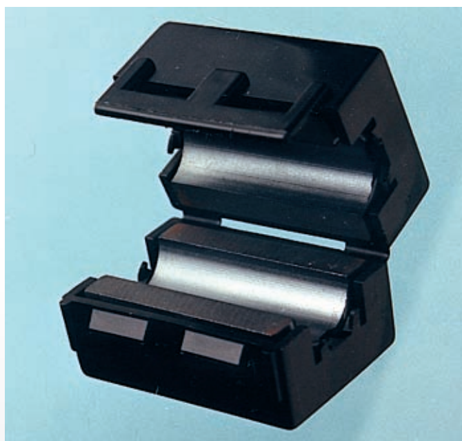
● Clip on ferrite filters can prove very useful – especially in dealing with interference FROM TV receivers and computers (see text).
