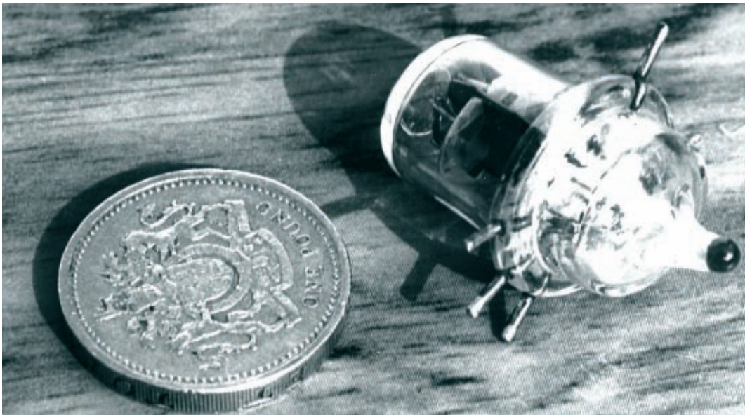
● Fig. 4: The small size of a typical (955) Acorn valve may be judged from the pound coin.
