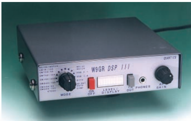
● Add-on digital signal processing (DSP) filters can help overcome many noise sources...whether they originate from within the home or off the air (see text).
