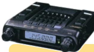
50 watt 2m FM mobile with DTMF mike and CTCSS making it ideal for internet linking (See [www.g7wfm.co.uk](http://www.g7wfm.co.uk) <<http://www.g7wfm.co.uk>> for details on internet linking)
