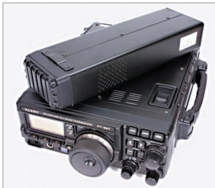
● The FT-897 with the optional automatic antenna tuning unit detached. The easy-carry 'rubberised' handle can be seen on the right.
