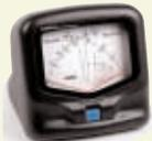
Two cross-needle VSWR/PWR Meters ideal for any shack. \*AV-20 3.5-150MHz \*AV-40 144-470MHz \*FWD/RFLD VSWR + PWR \*150W \*Sockets SO-239 \*50 Ohms \*Size 85x87x95mm \*Weight 280g
