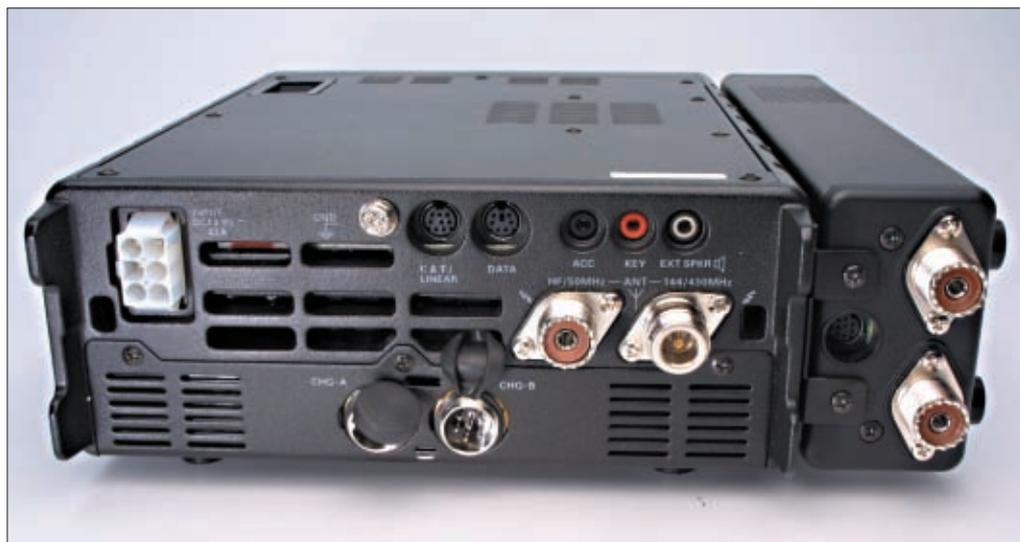
● Rear panel view of the FT-897. This transceiver provides portable 'Amateur Radio in one unit' from 1.8 to 430MHz, with many built-in features. You don't even have to carry a keyer for c.w. use...as it comes complete with a built-in version!
