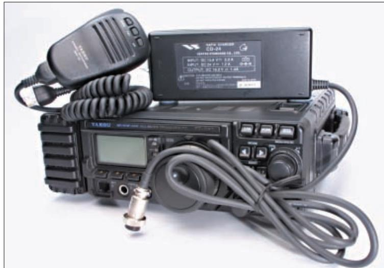
● Microphone and rapid charger unit and interconnecting leads.
