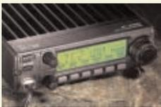
2m 55W FM mobile. Commercial grade, rugged construction. One piece die-cast aluminium chassis. Selectable green or amber display.
