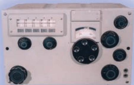
● Fig. 3 (Above): The Marconi HR110 receiver. The door above the tuning dial gives access to the crystal for fixed frequency operation (see text).
