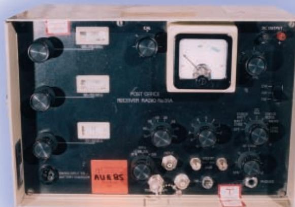
● Fig. 4: The Eddystone 31A receiver with the three tuners visible down left side, with the attenuators and mode switch at bottom centre (See text).
