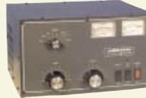
Ideal 600W HF Linear more than enough for the full UK limit. 160-10m including WARC bands. Uses 3x 811A low-cost valves. Matches all modern 100W solid state HF rigs. Silent running cooling fan.
