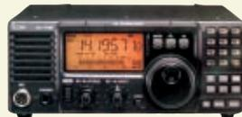
HF 100W transceiver. Covers all HF bands plus wideband receive. C/w auto notch, dual VFO, SWR meter etc. Options include extnl ATU DSP & filters.
