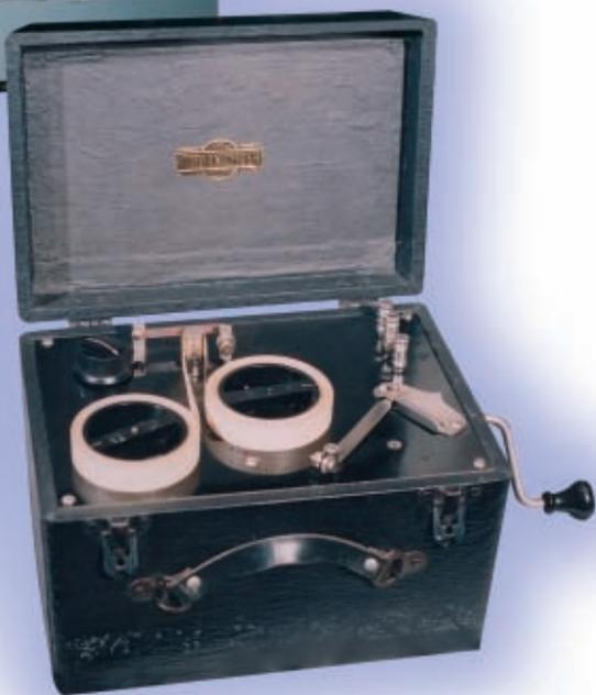
● Fig. 5: This really is a Morse wind up photograph! The Morse tape sender, and reel of paper tape with clockwork motor drive (See text).
