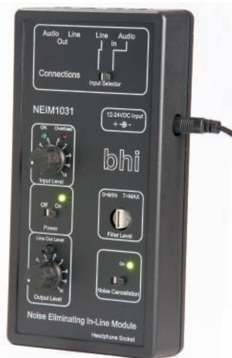
● Fig. 1: The bhi NEIM1031 in-line noise elimination module. The unit is operated from an external 12 to 24V d.c. input, and can be conveniently operated from the shack 13.8V supply. Power is applied (top right) via the ubiquitous female coaxial plug-in sockets we're so familiar with nowadays. The centre connection is the positive connection.
