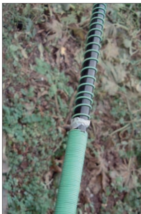
● Fig. 1: The top three metres of the roach pole are wound with a turns pitch of 12-13mm, and the lower two metres are close-wound with wire. This is the change over point. Note the use of masking tape to hold the wire temporarily in place.
