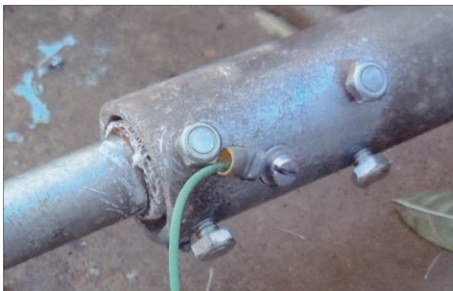
● Fig. 2: The alloy joining tube fitted into the top of the scaffold pole, using four clamping bolts. The alloy tube has been strengthened with wire mesh and car body filler.
