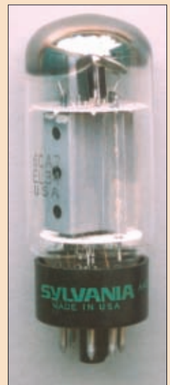
● Fig. 5: Mullard EL34s were always true pentodes, but the American valve shown here is labelled Sylvania - is a beam tetrode (See text).
