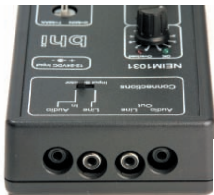
● Fig. 2: The mono audio input (switchable to either the phono or jack sockets) is provided with both an RCA phono and a 3.5mm jack socket. The audio line output (right) on the NEIM1031 is similarly equipped with a RCA phono socket and 3.5mm jack socket but does not incorporate switching (see text). Note: This end of the unit is referred to as the 'rear' within the bhi information booklet.
