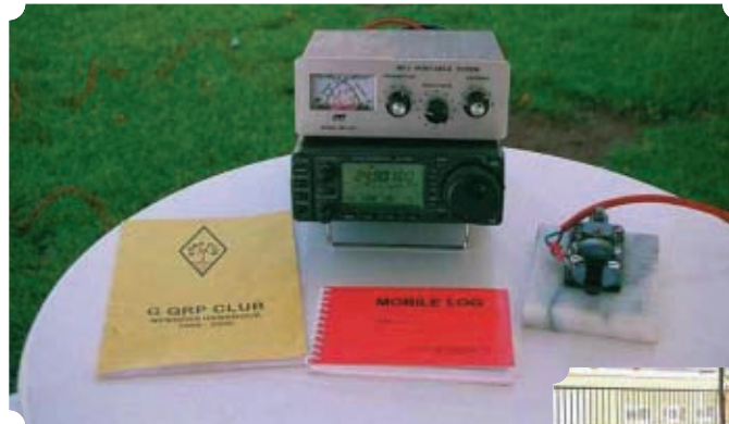
● The equipment, consisting of my Icom IC-706 together with a new SEC-1223 switch mode power supply.
