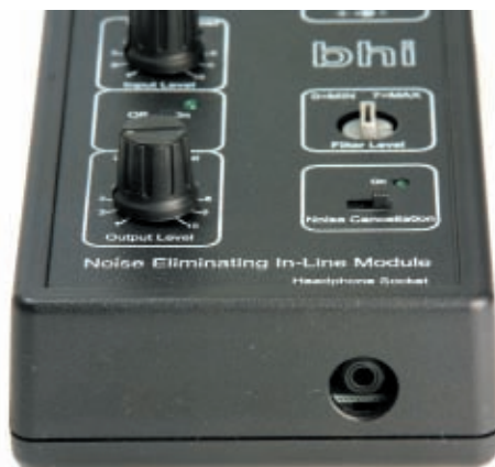
● Fig. 3: The 3.5mm headphone socket on the NEIM1031 is recessed, at the opposite end to the input/output connections (see text).
