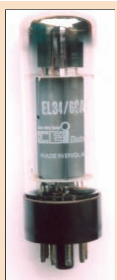
● Fig. 4: A Mullard-manufactured (but labelled CEI) EL34/6CA7 (see text).
