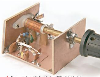
The prototype Permeability Tuned Oscillator (PTO) built 'Ugly' style by G3RJV. George says he found it to be "surprisingly stable" and urges readers to try the technique.
