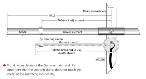
between the brass rod, the ptfe dielectric and the stainless steel shorting clip. The end of the gamma rod is clamped to the driven element 100mm from the centre line of the main boom. The spacing between the rod and the driven element is set at 30mm by the stainless steel fixing clamp (see **Fig. 4** for more detail).
