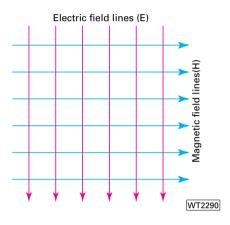
Fig. 1: (a) Once in the far field, the electric field (E) and the magnetic field (H) of a radio wave keep in phase while travelling at right angles to each other and at right angles to the direction of wave travel at a velocity of 300 metres per millionth of a second. (b) Elementary impression of a wave front approaching an observer. Since the polarisation corresponds to the vector of the electric field, the wave illustrated is shown to be vertically polarised.
