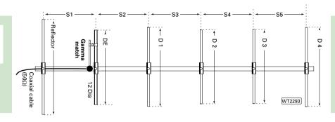
the coaxial cable feed line (which can degrade the beam polar pattern) since it is an unbalanced system.
