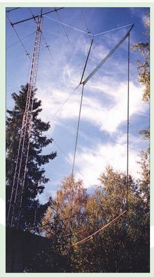
ome years ago when a VK friend and I were experimenti ng intensively with small antennas, it became clear to us, that for more accurate comparisons, we need a fixed reference antenna. The horizontal length of such reference antenna should be somewhere between full size  $(\lambda/2)$ and really short  $(\lambda/20)$ . Study of the antenna books showed that a loop having horizontal side length of around λ/8 could be an optimum compromise between radiation resistance (R<sub>r</sub>) and
