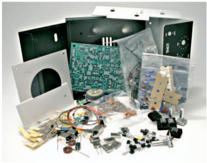
■ The Ten-Tec 1340 7MHz transceiver kit as supplied. The sturdy ready-painted steel case acts as storage box for the components and everything is clearly identified by the high quality manual. The main printed circuit board (p.c.b.) is silk screen over-printed with component placement locations (see text). The completed kit weighs just over 1kg (2.25lbs) and measures 70 x 152 x 152mm (HWD).
