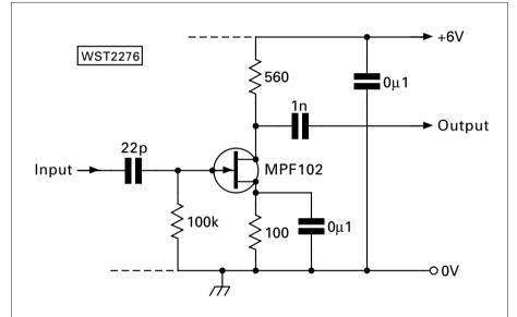
Fig. 2: For most applications a buffer amplifier will be required. The buffer amplifier, shown here is simple and George G3RJV found it improved the long term stability of the oscillator (see text).
