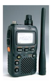
Close-up front view of the Yaesu VX-2E, showing the large l.c.d. main panel and the prominent easyto-use main rotary encoder (see hand-held transceiver is exactly what it says; a hand-held two-way radio and this takes me back a bit! Do you remember the old fashioned talking bricks? They were huge devices that with two hands you could just about manage to hold, as long as you had the muscles of Charles Atlas or some other muscle bound weight lifter!
