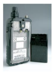
With the battery pack removed the VX-2E's robust diecast chassis/heat sink can` be seen.
