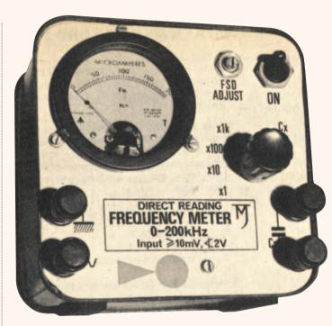
The Direct Frequency Meter taken from an electronically scanned photograph of the original project from the PW archives.
