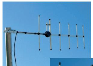
Fig. 2: The gamma match bar is covered in ptfe making a capacitive contact through the clamp to the
