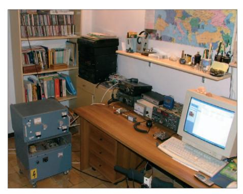
Anto IK4PMB (JN54) was active on the 144MHz band during the aurora on October 29. Equipment from left to right: 8877 1kW amplifier, Icom IC-735 transceiver, Icom IC-275H transceiver and Yaesu FT-225RD transceiver.
