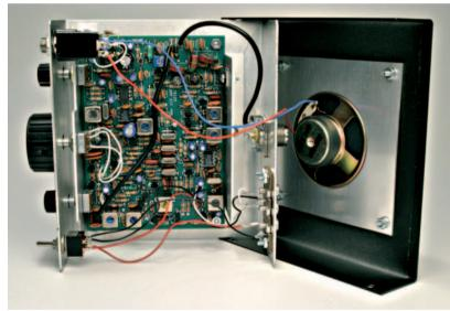
Photograph of the 1340 transceiver kit as completed by Kevin Nice G7TZC. The controls are mounted on an aluminium 'chassis' frame'. The relatively high density of the components on the p.c.b. can clearly be seen (see text).
