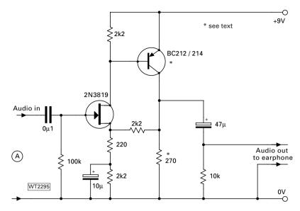
Simple circuit providing a high impedance input and a low impedance output. A small amount of
