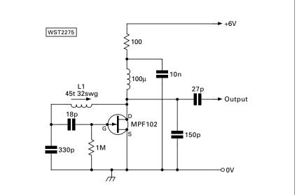
Fig. 1: The circuit of the PTO oscillator G3RJV tried. The circuit is based on the work of WA60TP work. In this example
