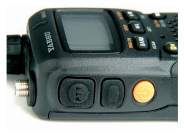
Although in effect a miniaturised transceiver, all the VX-2E's controls are conveniently positioned. The SMA antenna connector is seen (far left) with the main push-to-talk (p.t.t.) control immediately to its right (see text).
