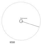
Fig. 2: From an isotropic source radio waves travel outwards spherically in empty space, progressively losing energy as they go.
