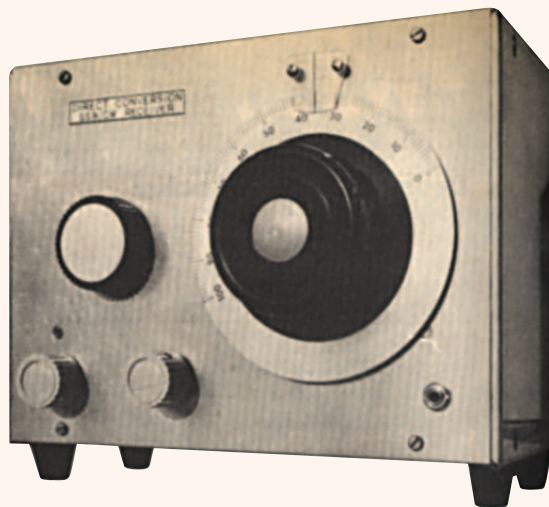
● Fig. 3: Archive drawing of the author's original project using an aluminium chassis. Modern alternatives for the aluminium chassis are available (see text).
