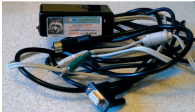
● The Rascal PSK31/RTTY interface was a particularly good find for Quentin GW3BV.
