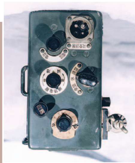
● Fig. 4: The Type 97 controls on the side of the case. The 4-pin socket is for the microphone-headset.
