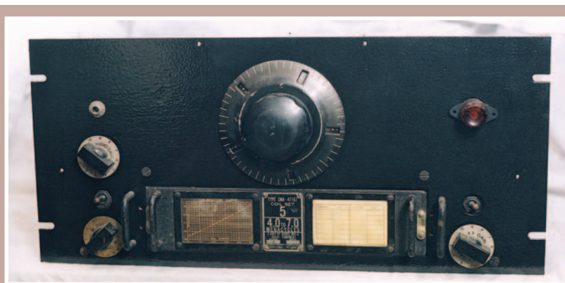
● Fig. 1: The HRO RBJ receiver, notice the absence of the S-meter and phasing controls. The coils are clearly marked RBJ-4 (see text).
