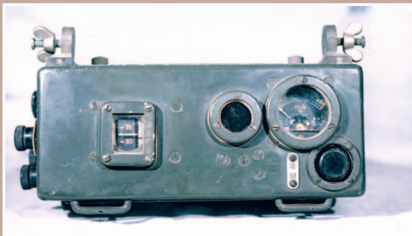
● Fig. 3: The Type 97 Japanese transceiver. Tuning window left, valve inspection window centre and p.t.t. button at the bottom right (see text).
