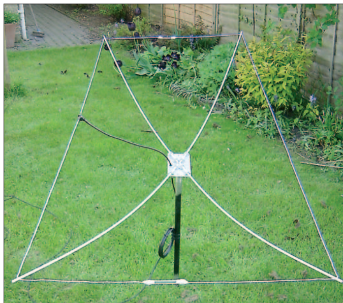
● The assembled wire Moxon Rectangle for 50MHz on its stub-mast, about to be installed 10m up on the roof. Note the upward tensioning curve of the g.r.p. spreaders and the location of the feeder together with its six-turn choke balun. The whole assembly weighs about 1.5kg.
