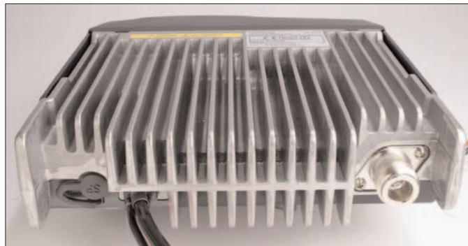
● Fig. 1: Close-up view of the massive heat-sinking for the 60W transceiver (see text).
