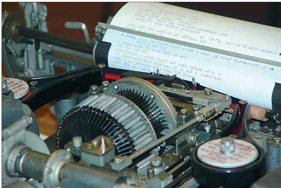
● Fig. 2: Close-up of the actual page of print produced from a Creed 7B teleprinter.
