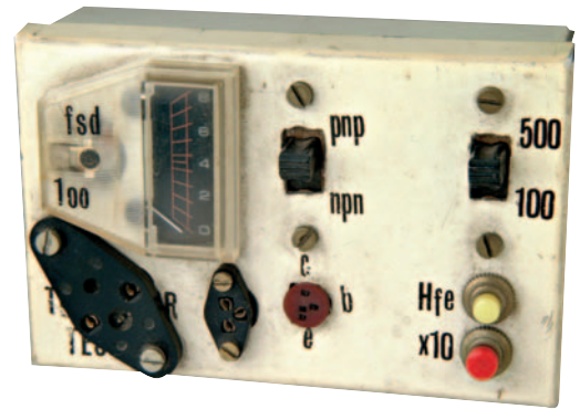
This transistor tester has provided G3RJV with over 20 years sterling service and George recommends that you build your own version this month!
