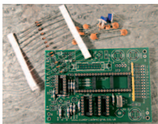
● Fig. 4: After the resistors, sockets and crystal have been fitted.
