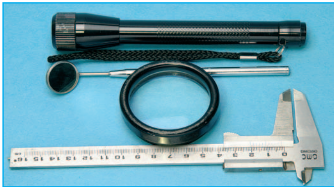
● Fig. 5: A good quality small torch is very useful, together with a dental inspection mirror and magnifying glass. Buying an Engineer's gauge will also help you get those internal and external measurements right!
