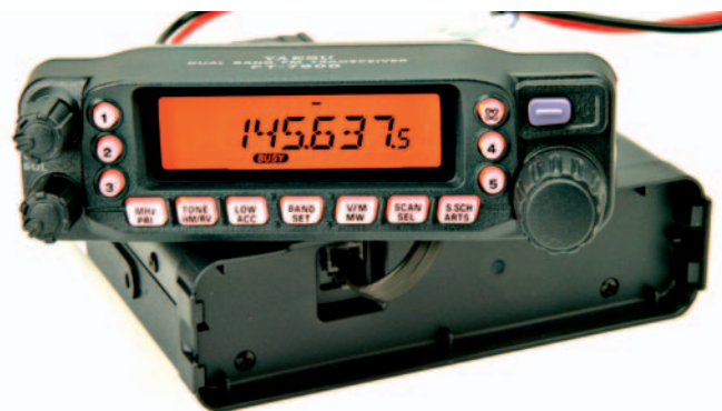
● Fig. 1: Showing the detachable control head which is removable for easier mounting (see text).
