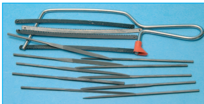
Fig. 4: Buy the best quality files you can afford, and ensure you have a good selection of round, half round, triangular and flat section types. A simple 'Junior' hacksaw is suitable for most light work.
