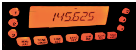
● Fig. 4: Having connected his d.c. supply to the FT-7800E, GOSKR was surprised by the warm orange-red glow from the buttons and the display panel. John found that the visible area of the display, though only 17 x 65mm, is very clear and easy to read.
