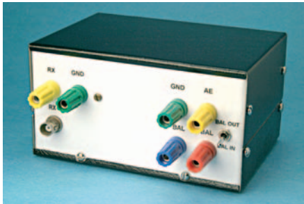
● Fig. 7: The back panel showing the BNC socket rather than the more common SO239.
