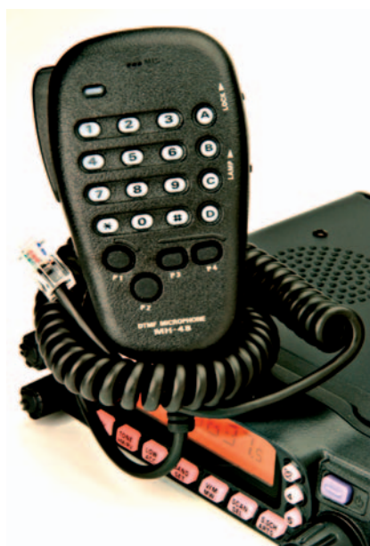
● Fig. 5: The review model was supplied with MH-48 DTMF Hand Microphone which made the operation of the unit extremely easy. The v.f.o. frequencies can be entered directly to the display, from the numeric keypad (see text).
