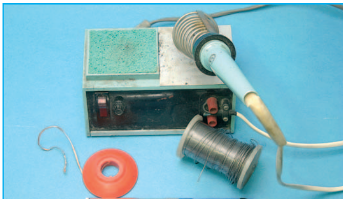
● Fig. 6: A heavy duty soldering station (the example in photograph is British made) is an excellent investment. Desoldering wick (the orange disc) and a desoldering pump are also extremely useful (see text).
