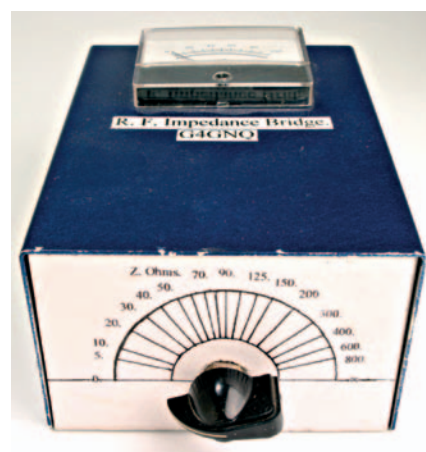
● Fig. 3: Geoff G4GNQ temporarily attached a card to the front of the case, so the scale could be calibrated (see text).
