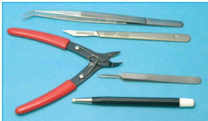
Fig. 3: Small cutters, tweezers, scalpels along with fibre-tipped pens (for cleaning contacts, etc.) are extremely helpful. Although more expensive, reverse action (you squeeze to open them) tweezers are very useful for heat shunting while soldering) and are highly recommended.
