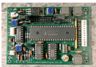
● Fig. 5: The main board assembled, now to tackle the l.c.d. fittings assembly.
