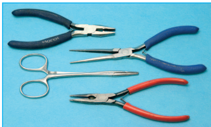
Fig. 2: A good choice of quality pliers and forceps is essential for the workshop. Spring loaded types (the springs hold the jaws open) feel better in the hand and are recommended.
