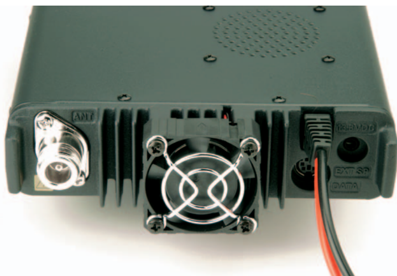
Fig. 2: The powerful cooling fan is almost silent when running. A single N type plug is provide for v.h.f./u.h.f. use. The data input socket (see text) is directly under the power input entry point, with the external loudspeaker socket to the far right (see text).
