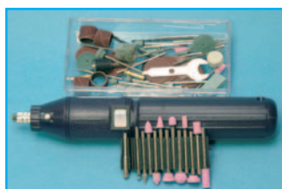
● Fig 7: A battery powered rotary grinding/drilling tool with a comprehensive set of tools, such as this can prove extremely useful in your workshop.
