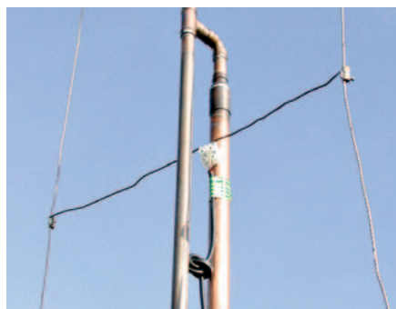
● Fig. 4: Detail of the construction method. The antenna is fed directly with 50Ω coaxial cable via a connector block and connected to the vertical wires by inserts from connector blocks. This enables the connection points to be adjusted for minimum s.w.r. See text for more detail.
