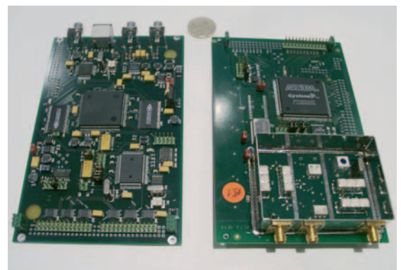
● The Digital ATV boards purchased by the BATC for trial and evaluation. Vision/Sound to MPEG2 encoder on left, digital modulator and transmitter on the right.
