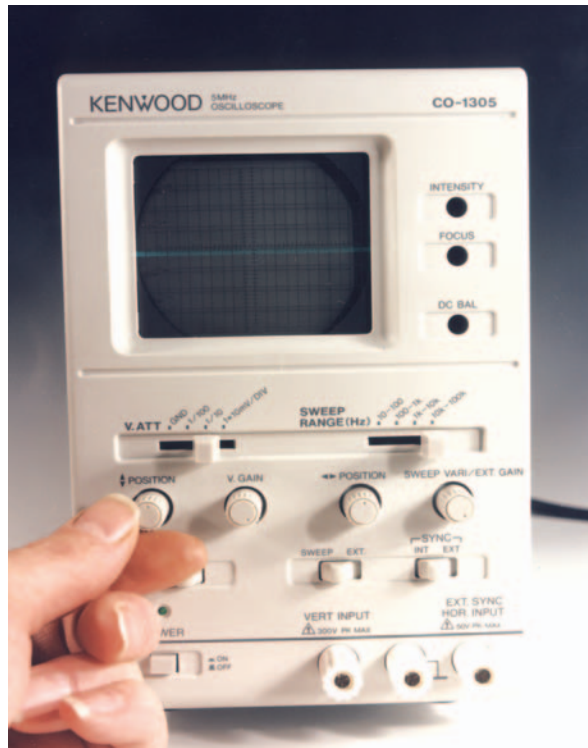
● Fig.3: This Kenwood CO1305 5MHz bandwidth single beam oscilloscope would credit any workbench. It's an ideal 'starter' instrument. It's attractive, easy-to-use and reliable.
