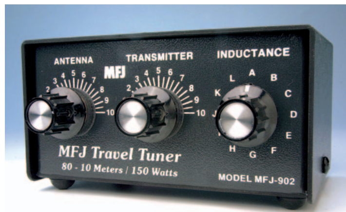
● The MFJ-902 Travel Tuner. It's small enough to be carried in the hand, works well with low power (QRP) and will cope just as well with high power.
