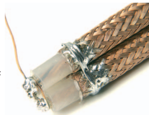
● Fig. 3: At the 'inner' ends the screens are soldered together. The inner conductors are connected together separately.
