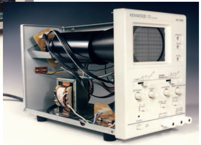
● Fig.4: The inside view of the Kenwood CO1305 oscilloscope. It may look deceptively simple but the clean lines and use of neat printed circuit boards somewhat 'play down' what the instrument can achieve in the workshop. The c.r.t. itself is housed within the large black screening sheath which extends to the flared out section of the tube (to the right). The screening sheath limits the effects of external electrical signals (that could effect the displayed trace) and also any radiated signals from the instrument itself.
