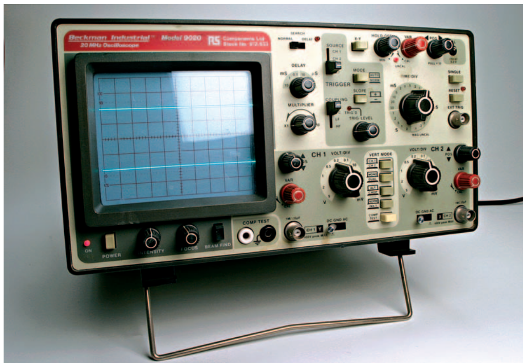
● Rob Mannion G3XFD tries really hard to persuade you not to be overawed by a modern oscilloscope. Rob says "Don't be put off by the apparent complexity". Instead, he says it can be a powerful friend on the workbench. This photograph shows a Beckman Industries 20MHz bandwidth 'scope.
