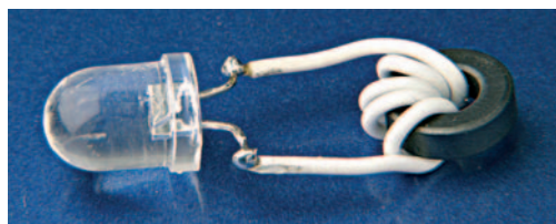
● Fig. 1: A modern r.f. 'sniffer' (above) and circuit (below) using an ultra-bright or super-bright l.e.d. to indicate the amount of r.f. current passing through a wire. This is a modern version of the bulb-in-line system for providing an indication of r.f. current flow (see text).
