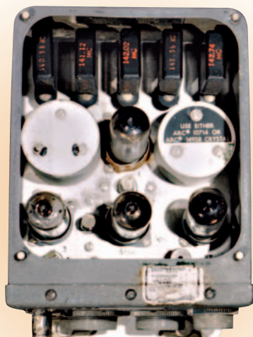
● Fig. 5: Inside the T-13. Four 5763 valves are used and the unit still has its 142MHz crystals fitted (see text).
