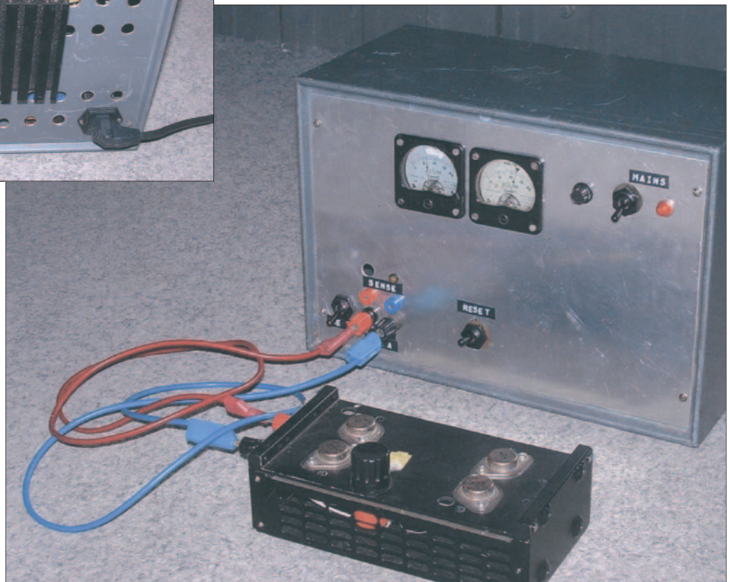
● Fig. 6: Testing the prototype high current p.s.u. using an electronic loading 'resistor' consisting of four power transistors.
