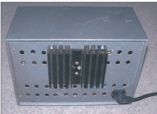
● Fig. 5: The heat-sink and ventilation holes are visible in this view of the rear panel of the project (see text).
