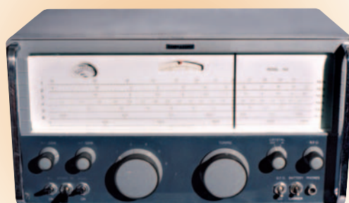
● Fig. 1: The Eddystone 960 transistorised receiver, complete with large easy-to-read tuning scale (see text).
