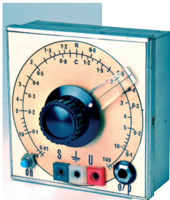
● “Here's one I built before” - George G3RJV describes the building and use of the AC Bridge - a simple instrument, which he thinks is very useful in the workshop.
