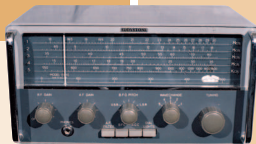
● Fig. 5: The Eddystone EC10 - much in demand as a tuneable i.f. v.h.f. down converters in the mid 1960s (see text).
