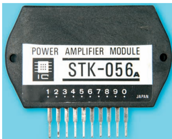
● Fig. 9: Incorporating both i.c.s and discrete transistors, some amplifiers offered up to 50W output with low distortion.
