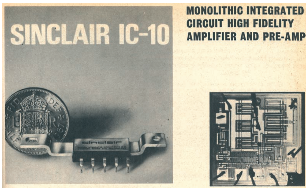
● Fig. 7: Photograph of Plessey audio i.c. and heat sink under its guise as the Sinclair IC-10.
